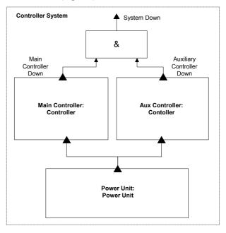
Fig. 3-3: The Component "Controller System"
