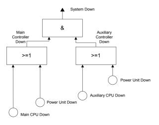
Fig. 2-1: Simple Fault Tree
