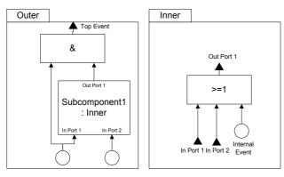
Fig. 3-8: Component-wise Fault Tree Decomposition
