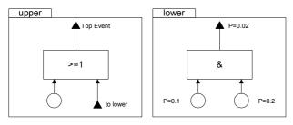
Fig. 3-7: Traditional Fault Tree Decomposition
