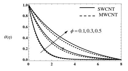
**Figure 3** Temperature profiles for different values of  $\phi$
