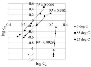
Figure 2: Fitting of the Freundlich isotherm model at various temperatures,  $C_0 = 2 \text{ mg/L}$
