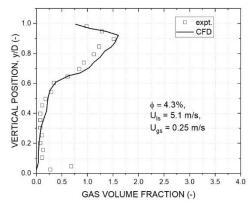
Figure 2. Gas volume fraction vs. vertical coordinate for the experimental and computed data
