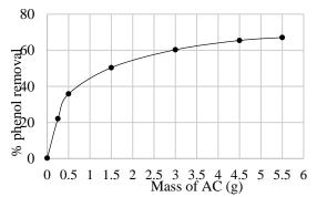
Figure 1: Relationship between mass of AC and the quantity of phenol removed;  $C_0 = 2 \text{ mg/L}$ ,  $T = 25^{\circ}C$
