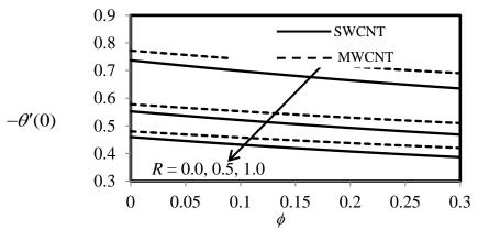
Fig. 5 Heat transfer rate verses volume fraction for different values of R
