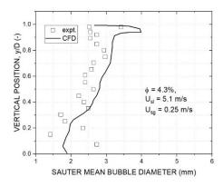
Figure 1: Sauter mean bubble diameter vs. vertical coordinate for the experimental and computed data
