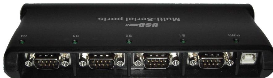
**Figure 3.5** USB multi-serial port adapter.
