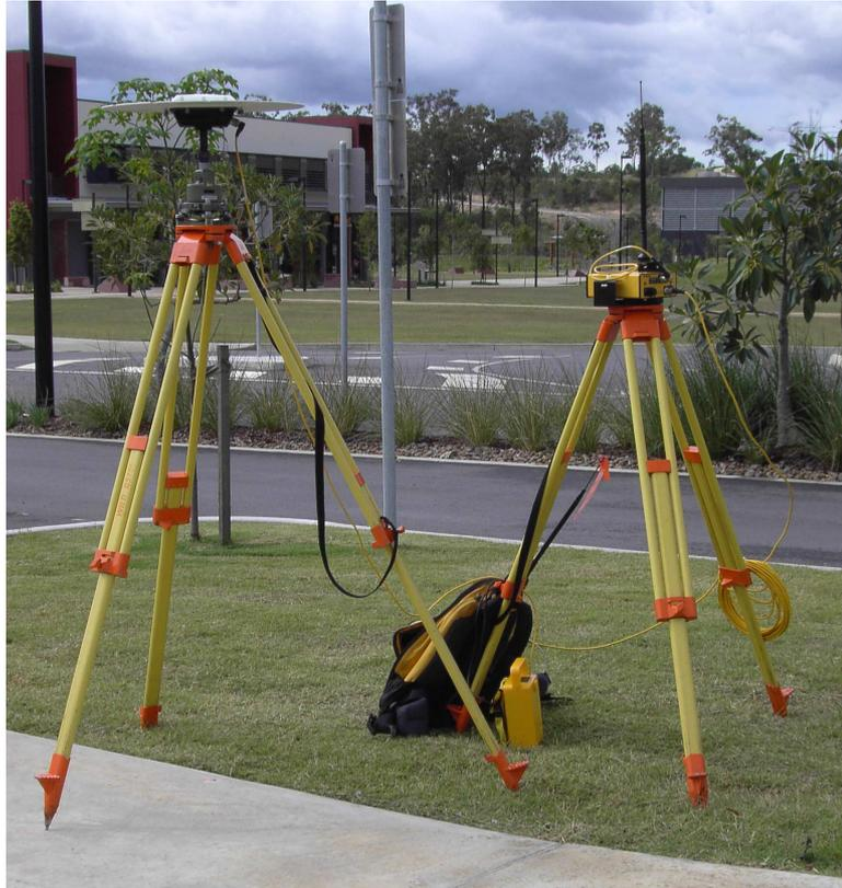
**Figure 3.9** Conventional RTK Base Station.
