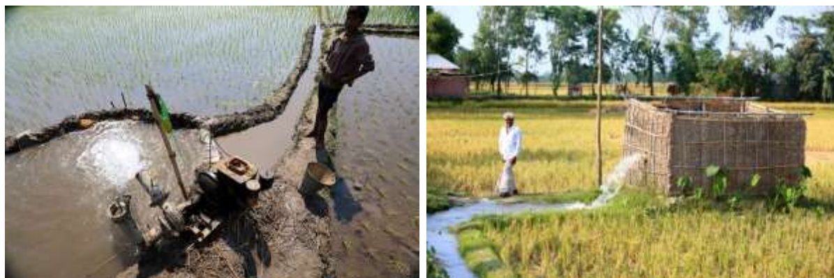
Figure 17. A diesel STW (left) and an electric STW (right)
