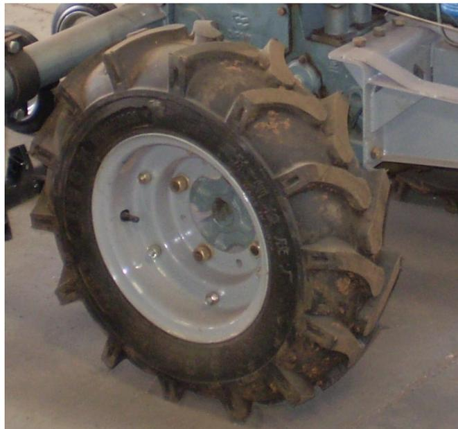
Figure 3.3: An illustration showing the standard pneumatic tyre for a power tiller.
