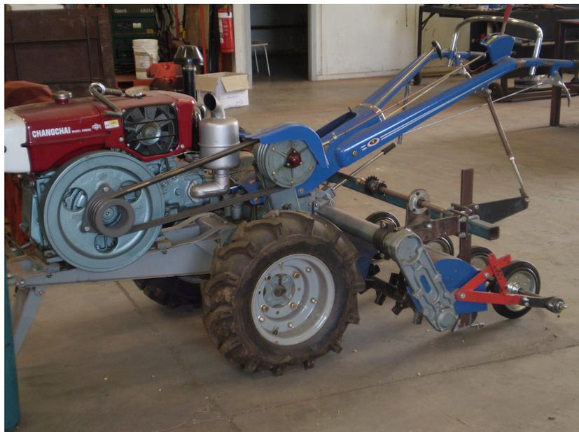
Figure 1.6: A power tiller with a rotary hoe attached.
