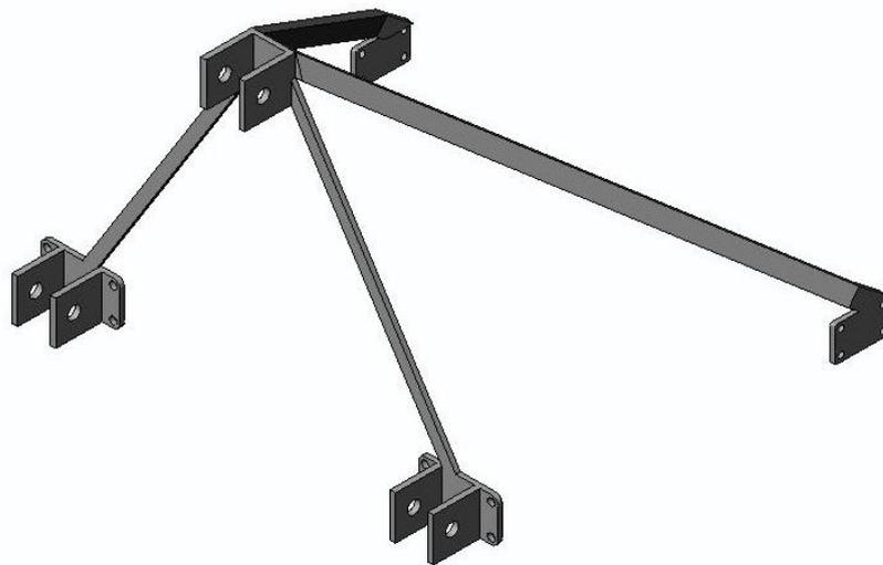
Figure 8.1: A basic design of a Three Point Linkage hitching system for the seed drill.
