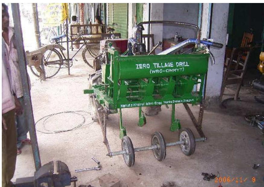
Figure 1.1: A modified version of the no till seed drill made by CIMMYT.
