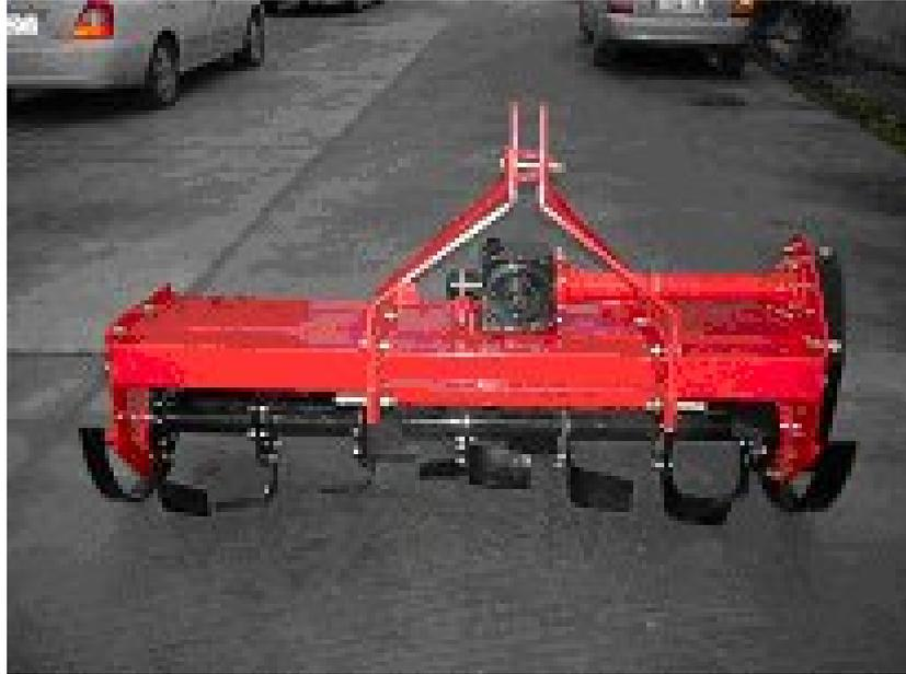
Figure 1.5: A typical rotary hoe designed for a small tractor.
