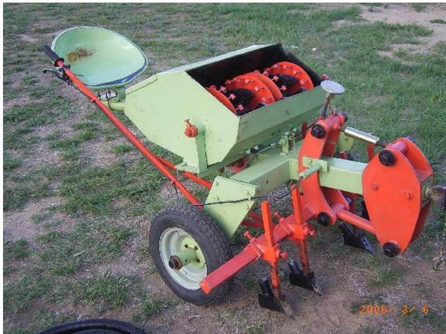
Figure 2.3: A cheap Indian made seed drill.
