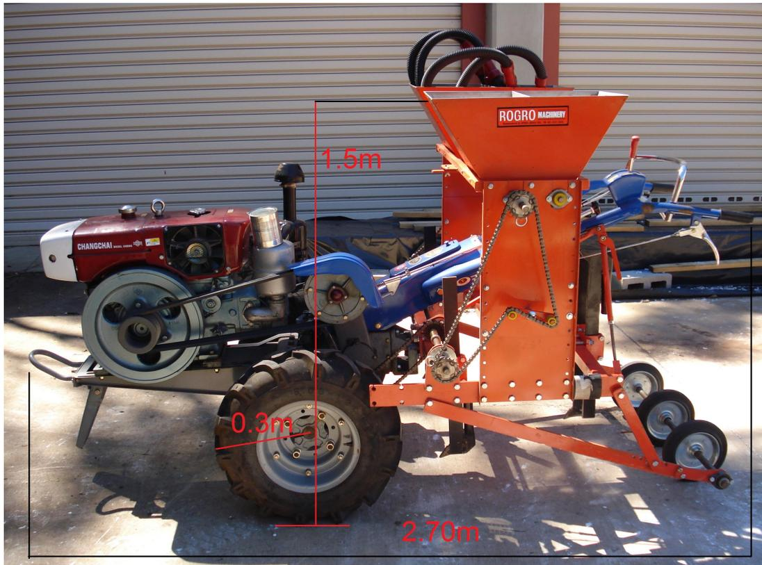
Figure 3.2: An illustration showing approximate dimensions of the power tiller and seed drill.
