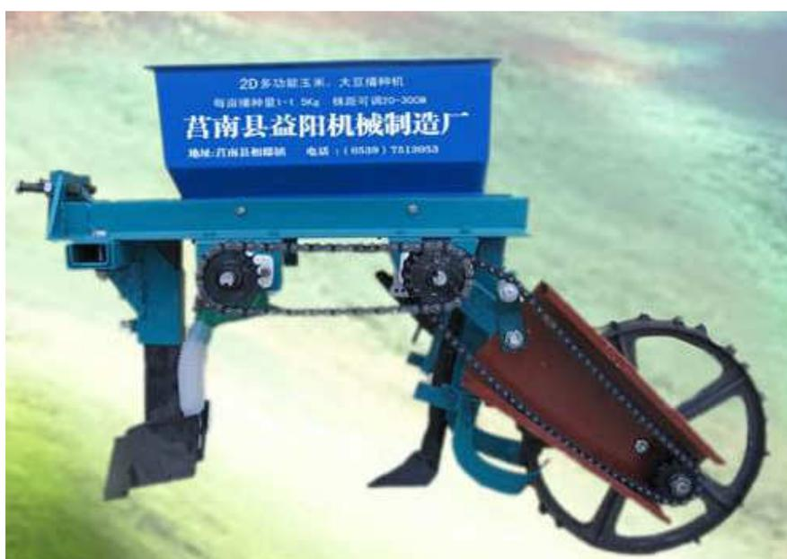
Figure 2.4: A Chinese made seed and fertilizer drill.
