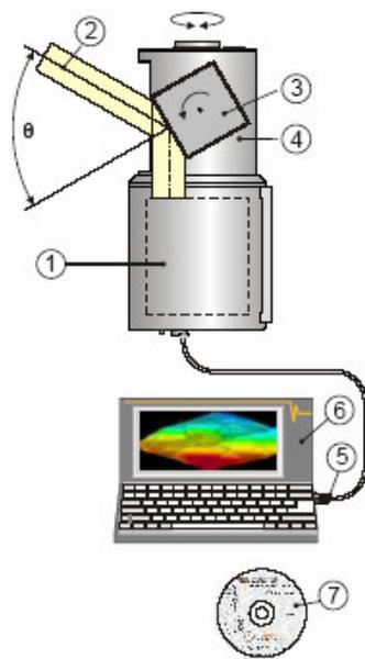
The range finder electronics (1) of the 3D scanner RIEGL LMS-Z210i is optimized in order to meet the requirements of high speed scanning (fast laser repetition rate, fast signal processing, and high speed data interface).
