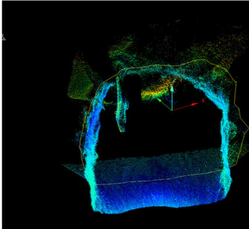
Figure 4.9: Voidworks screen capture of the loop wrap function. This function creates a polygon around the outermost points selected.
