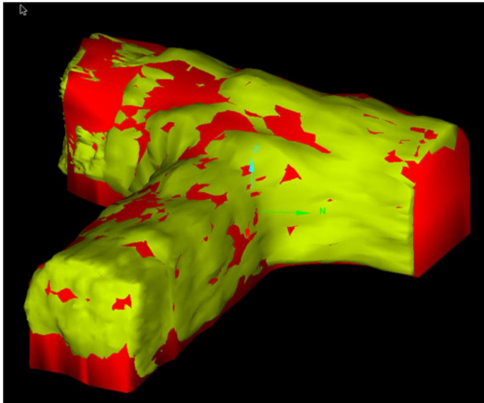
Figure 4.7: Voidworks screen capture of solid models of 280 Level drive surveys. The scanner data model is gold and the total station data is red.
