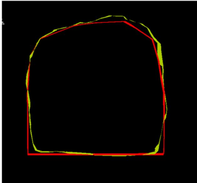
Figure 4.11: Voidworks screen capture of a cross-section of the two solid models of 280 Level C0 XC.
