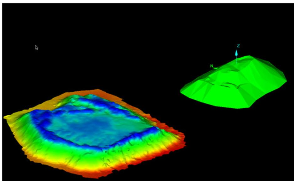
Figure 4.12: Voidworks screen capture of a surface stockpile. Notice the difference in detail between stockpiles
