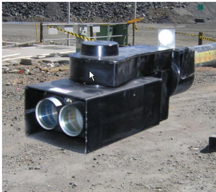
Figure 3.2: Photograph of the CMS head on the surface at Cannington mine.
