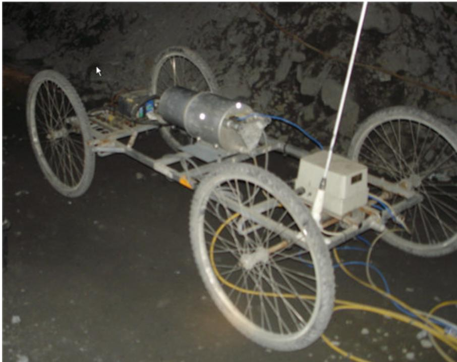
Figure 3.7 Scanner attached to the CMS trolley in the longitudinal position
