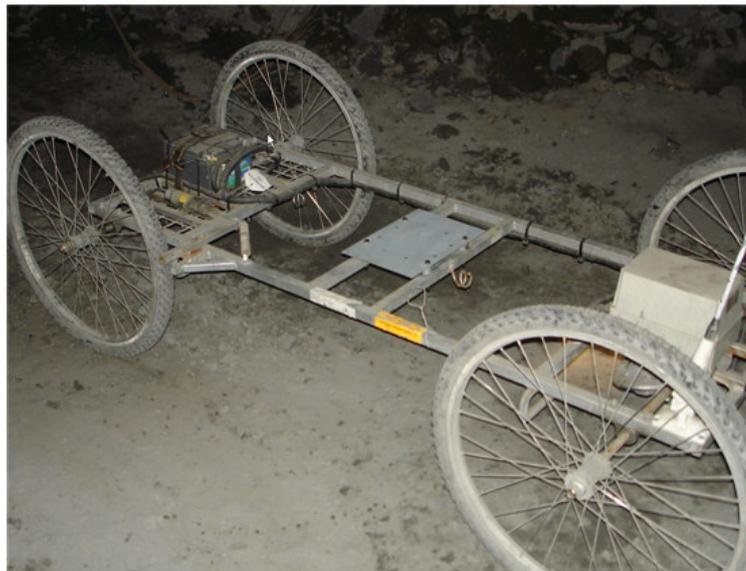
Figure 3.5: Photograph of the CMS trolley with scanner base plate attached
