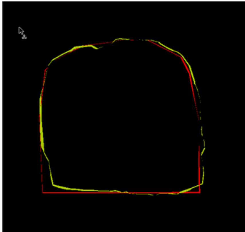
Figure 4.10: Voidworks screen capture of a cross-section of the two solid models of 280 Level C0 XC.
