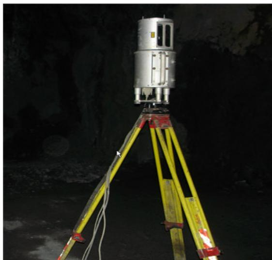
Figure 3.1: Photograph of the Riegl LMS-z210 underground at Cannington mine.
