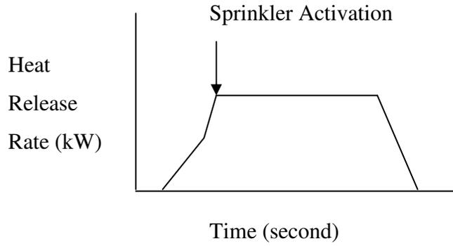
Figure 3: Sprinkler Control Mode
