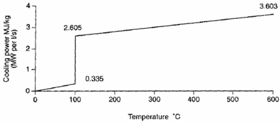
Figure 4: Cooling power Of Water
