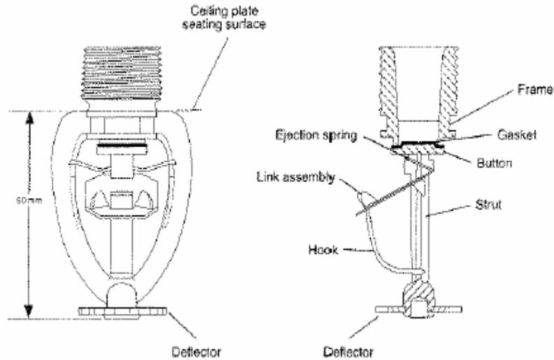
Figure 6: Typical Sprinkler Heads
