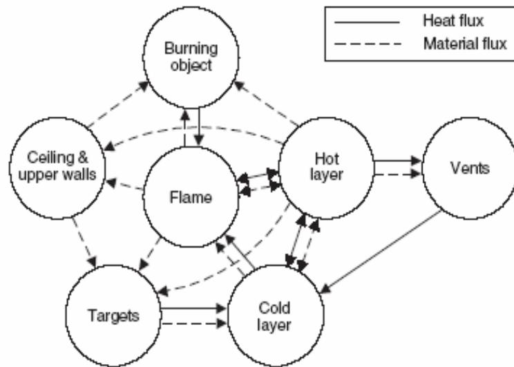
Figure 2: Interactions Of The Compartment Of A Room Fire Model;
