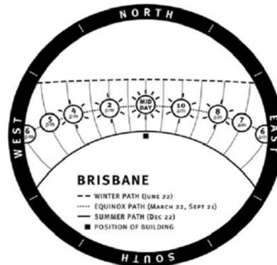
Figure 12: Brisbane Sunpath Diagram
