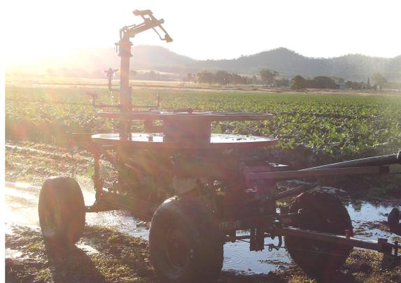
**Figure 2.3: Trolley-winch irrigator after use**
