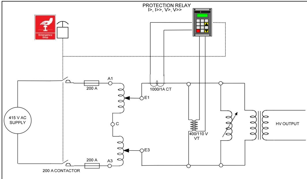
**Figure 5.1:** Simplified schematic of Power Supply
