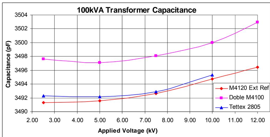
**Figure 6.4:** GST Capacitance test result comparisons for 100kVA Transformer.
