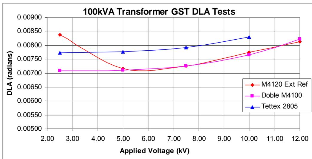
**Figure 6.3:** GST DLA test result comparisons for 100kVA Transformer .
