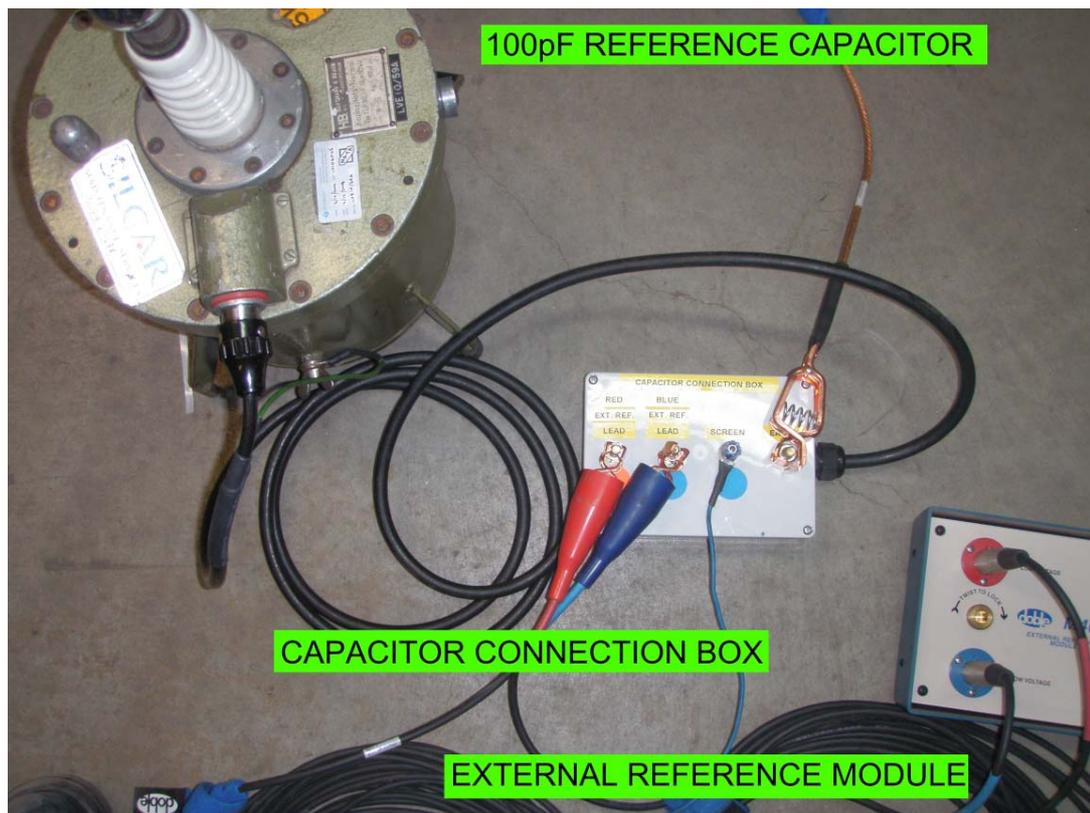
**Figure 5.7:** Measurement Equipment
