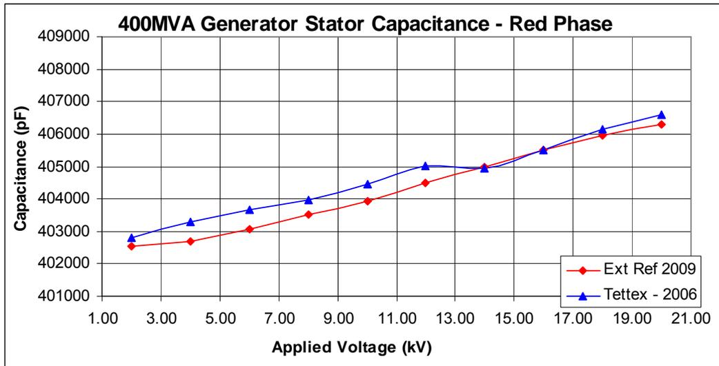
**Figure 6.8:** GST capacitance test result comparisons for a 20kV 400MVA Generator Stator – red phase winding.
