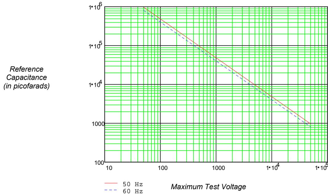
The maximum allowable test voltage is limited by the rating of the External Reference Capacitor, or by the voltage capability of the available external source, provided the criteria for maximum allowable reference current is not exceeded.
