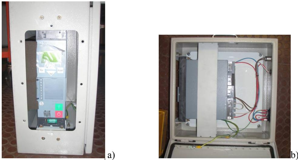
**Figure 5.5:** Relay Box. a) Front view b) Side view with lid open
