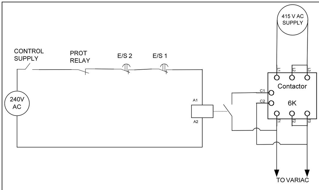
**Figure 5.2:** Simplified schematic of the contactor control circuit
