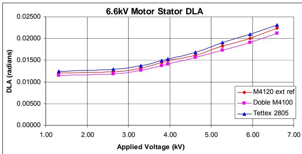
**Figure 6.5:** GST DLA test result comparisons for a 6.6kV Motor Stator – white phase winding.
