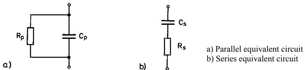
**Figure 2.1:** Equivalent circuits for a dissipative dielectric for alternating voltage (Kind 1978, p. 56)
