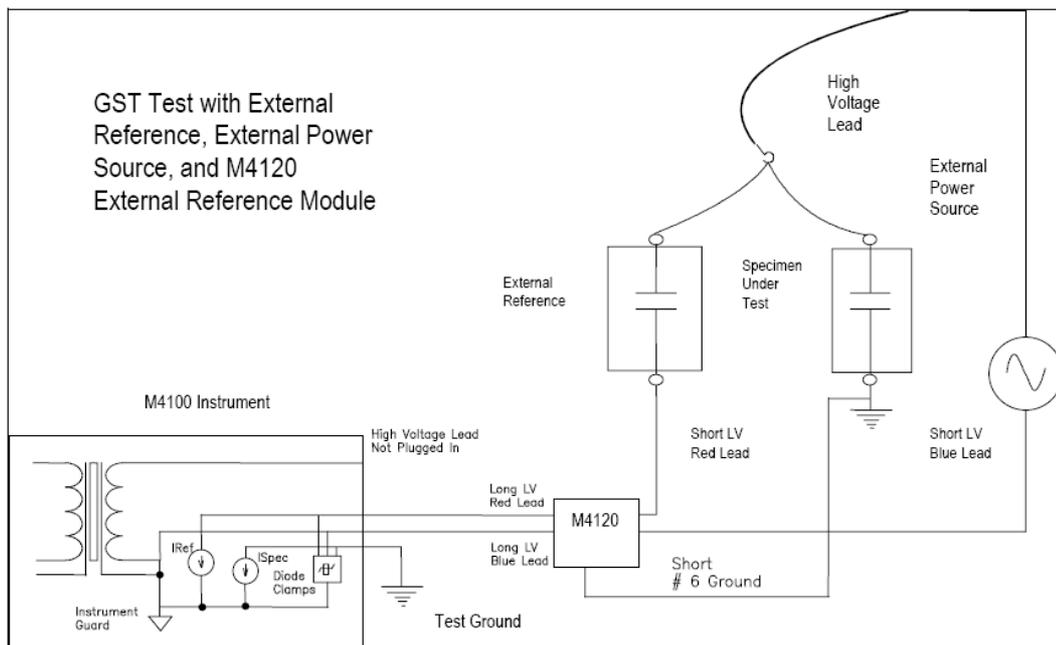
**Figure 5.8:** GST Test setup (Doble M4120 Application Notes, page 5)
