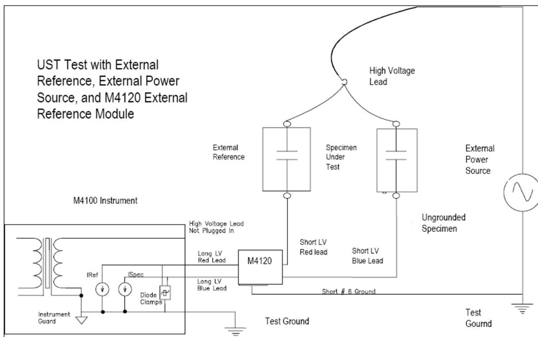
**Figure 5.9:** UST Test setup (Doble M4120 Application Notes, page 4)
