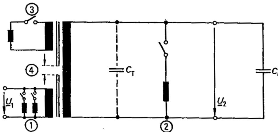
**Figure 2.5:** Methods for Compensation of the capacitive reactive kVA (Kind & Fresser 2001, p. 8)
