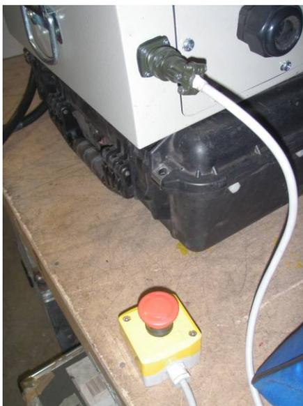
**Figure 5.4:** Emergency Stop plugged into contactor box.
