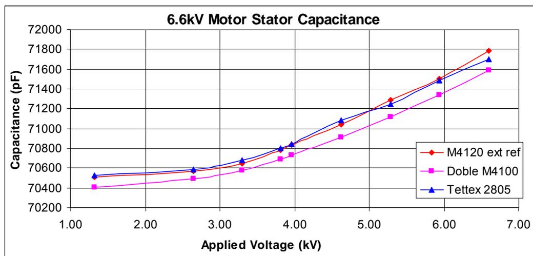
**Figure 6.6:** GST Capacitance test result comparisons for a 6.6kV Motor Stator – white phase winding.
