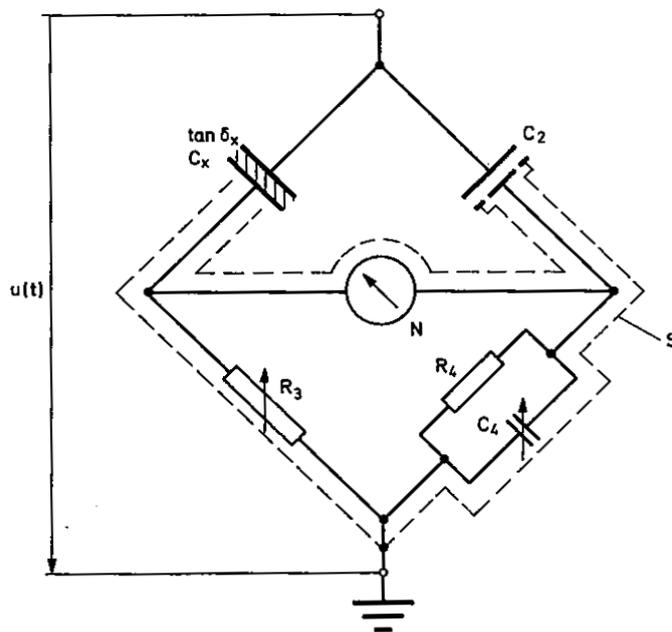
**Figure 2.3:** Circuit of the Schering Bridge (Kind & Freser 2001, p. 98)
