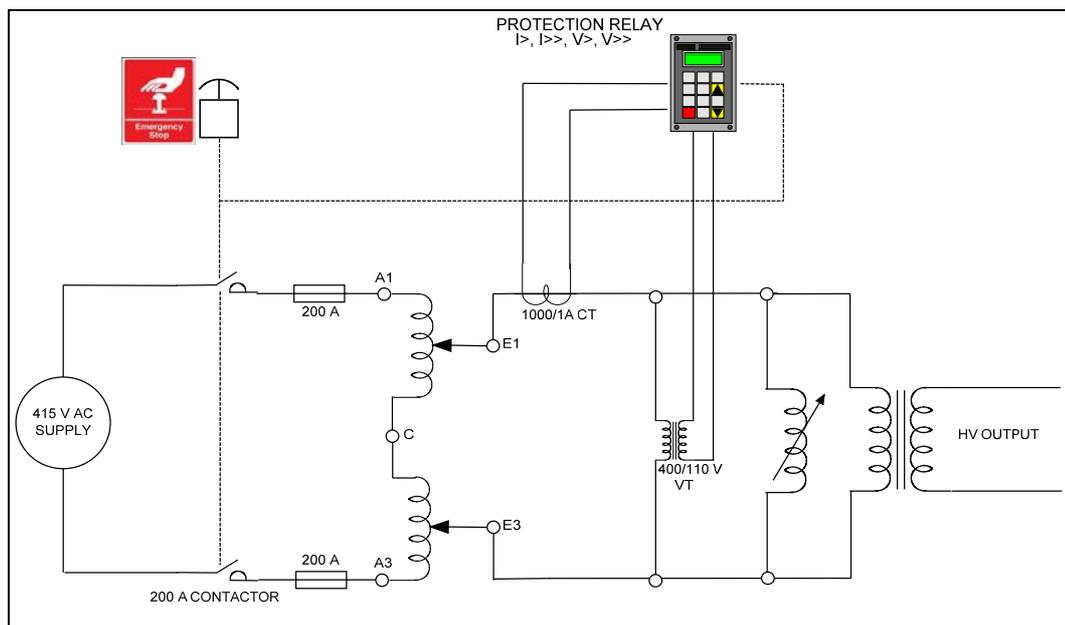
**Figure 4.1:** Simplified schematic of Power Supply Proposal A
