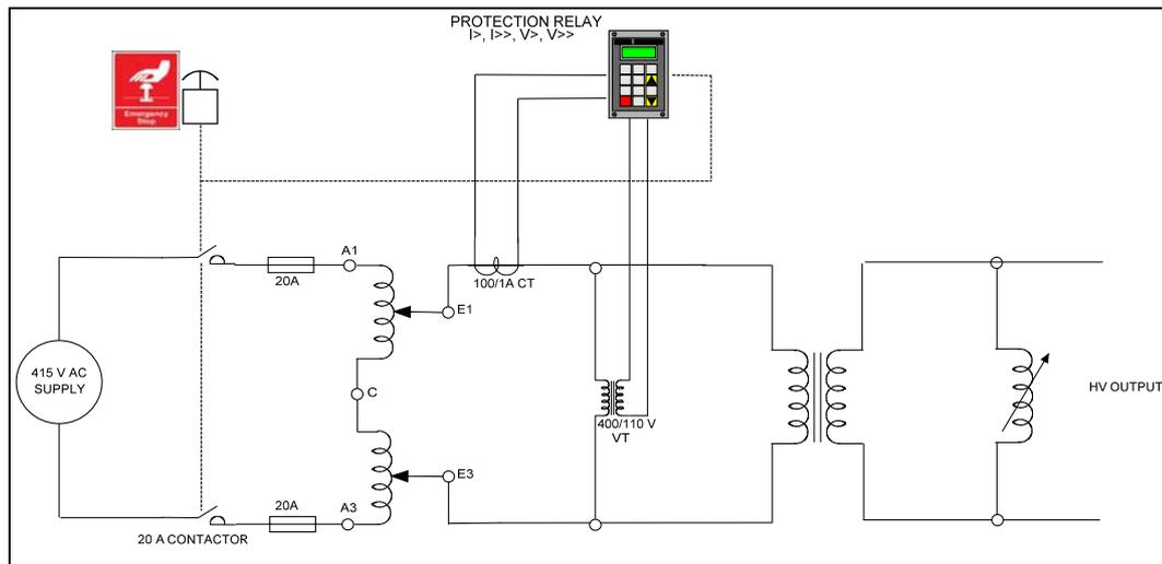
**Figure 4.2:** Simplified schematic of Power Supply Proposal B
