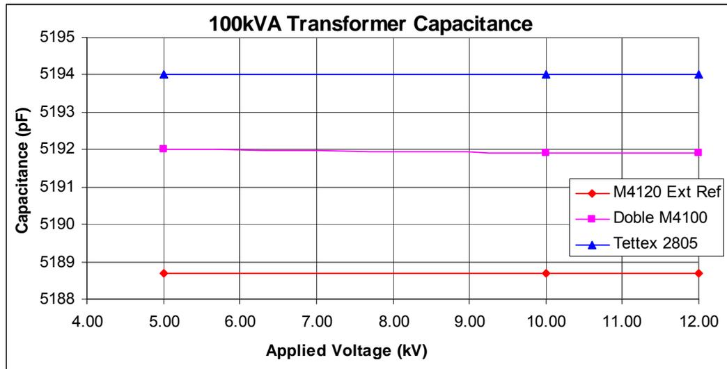
**Figure 6.2:** UST Capacitance test result comparisons for 100kVA Transformer.
