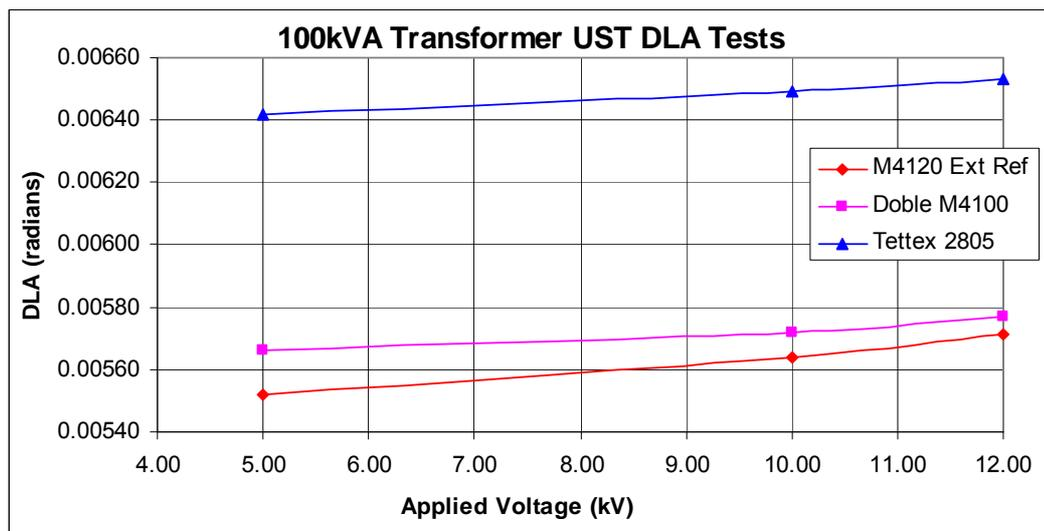
**Figure 6.1:** UST DLA test result comparisons for 100kVA Transformer.
