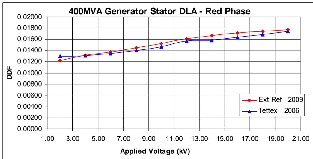
**Figure 6.7:** GST DLA test result comparisons for a 20kV 400MVA Generator Stator – red phase winding.
