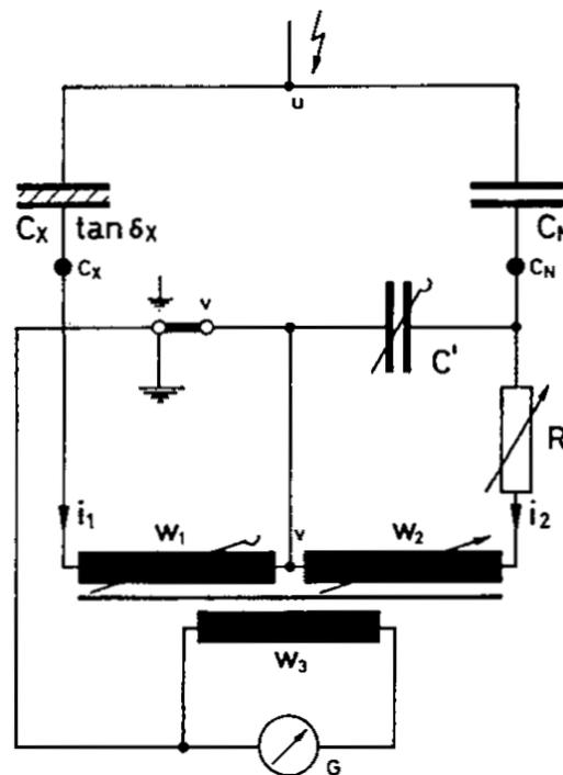
**Figure 2.4:** Tettex Type 2805 basic circuit (Tettex 1976, p. 11)
