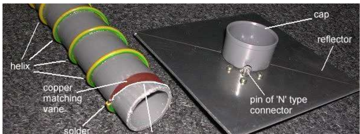
Figure 13 Almost finished helix antenna.
