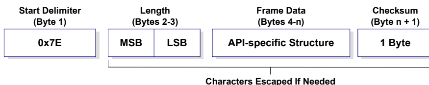
Figure 9-02. UART Data Frame Structure - with escape control characters:
