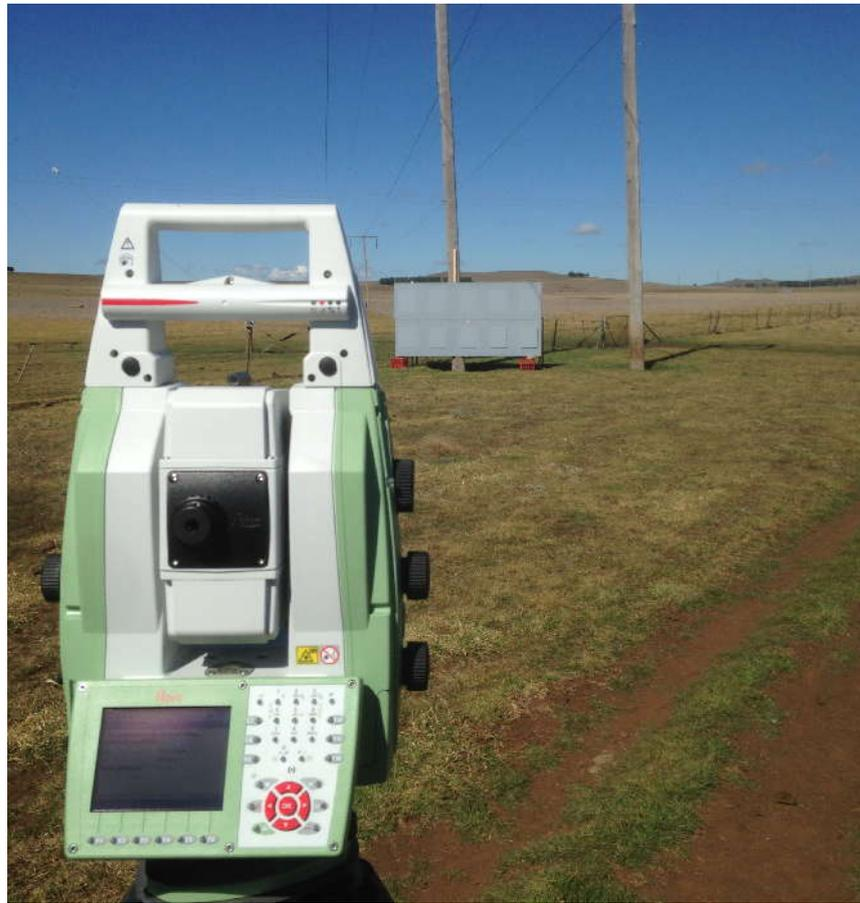
Figure 3.7 – Scanner and Target set up at 25m interval.
