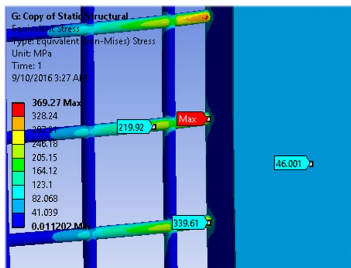
Figure 5-18 FEA Result of Wire Mesh Restraint Using Sheet Metal Seam
