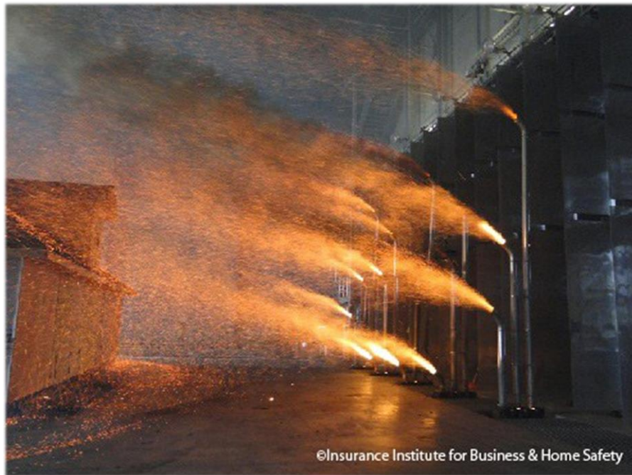
Figure 2-8 Image Showing a Simulated Firebrand Attack Upon a Dwelling (Insurance Institute for Business and Home Safety, 2016)
