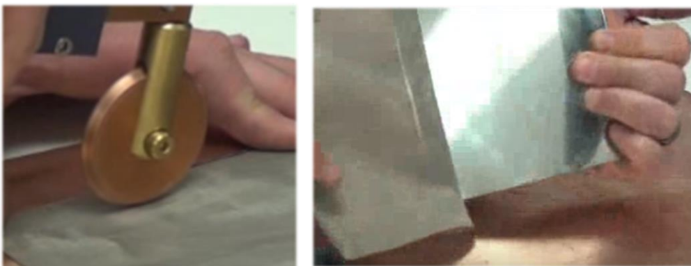
Figure 5-19 Pictures Showing Welding of Wire Mesh to Sheet Metal (Sunstone Engineering, 2015)
