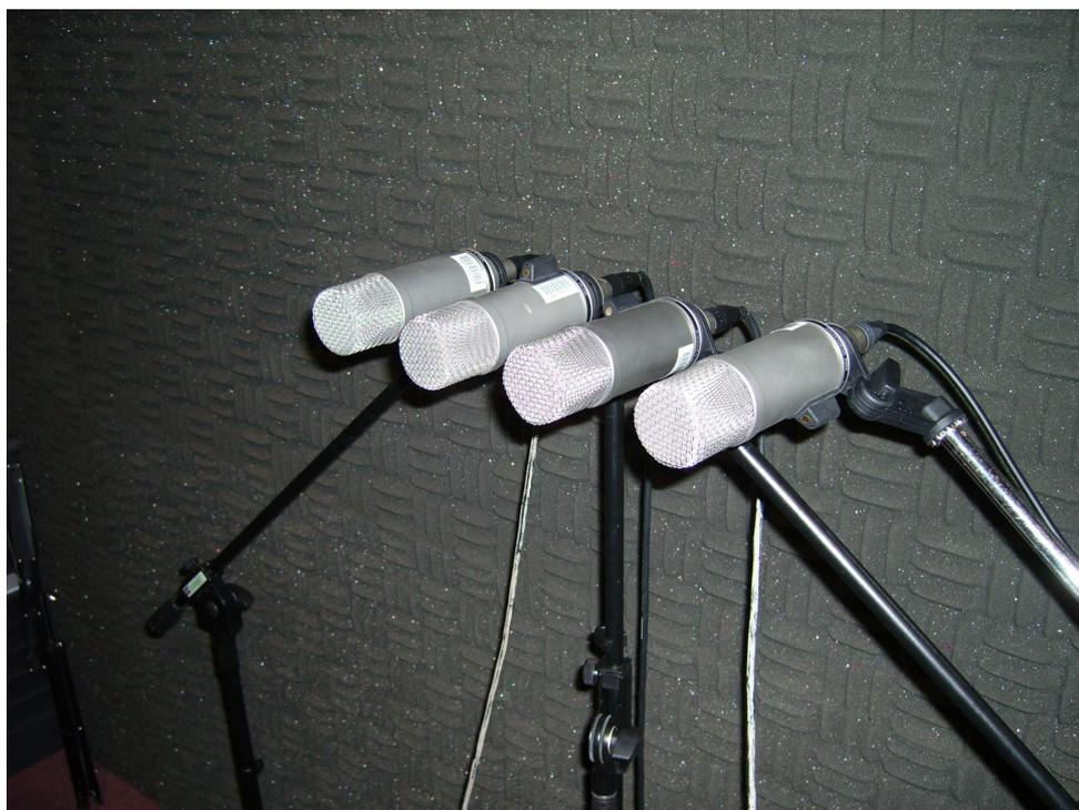
Figure 6.7: Experimental setup of a four element microphone array, spaced at  $0.1m$ .
