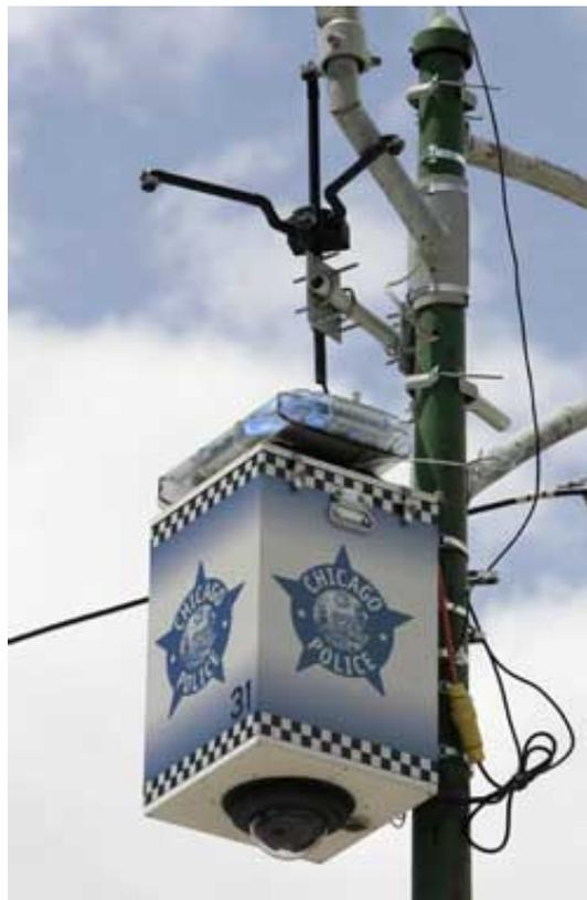
Figure 2.3: The SENTRI or Smart Sensor Enabled Neural Threat Recognition system attached to a phone pole in Chicago (Reichgott 2005, p. 1).
