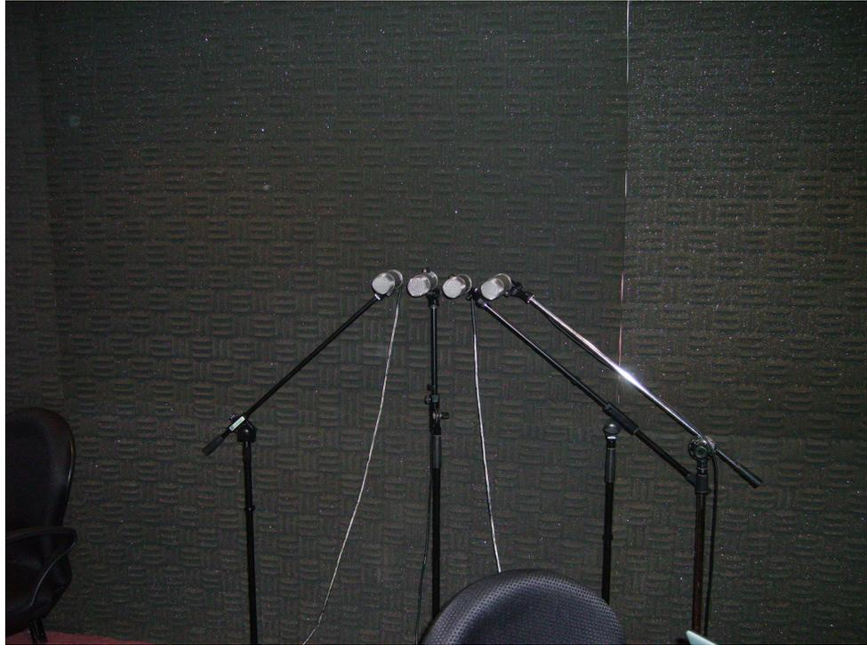
Figure 6.6: Experimental setup of a four element microphone array, spaced at  $0.1m$ .
