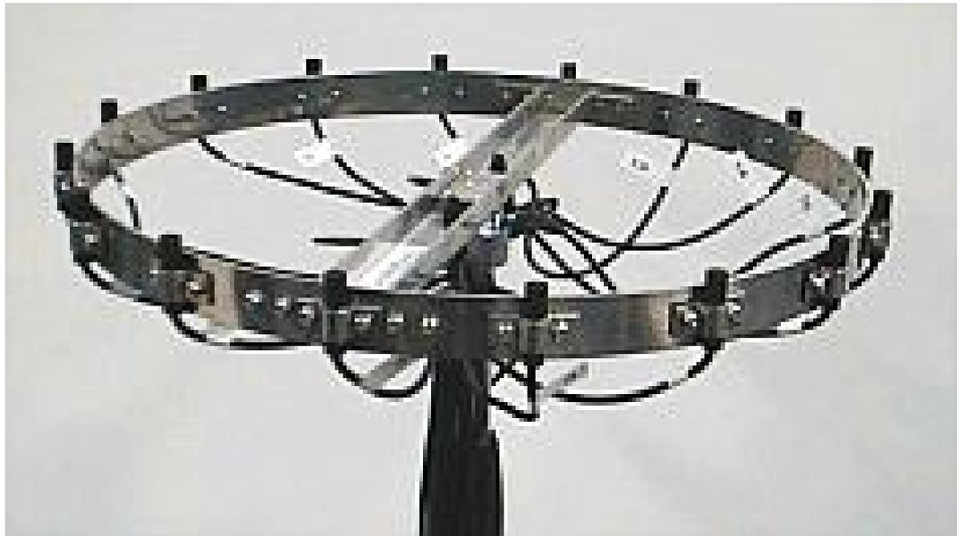
Figure 1.2: Microphones arranged in a UCA geometry (Hiyane & Iio 2000).
