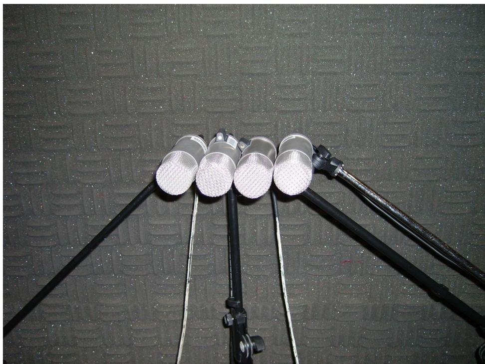
Figure 6.8: Experimental setup of a four element microphone array, spaced at  $0.055m$ .
