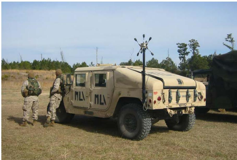
Figure 2.4: The boomerang system mounted onto a High Mobility Multipurpose Wheeled Vehicle (HMMWV) (BBN Technologies 2006, p. 1).
