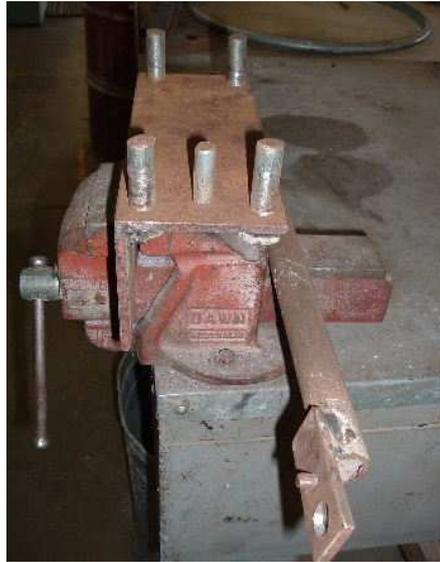
**Figure 4.2:** Bending Jig
