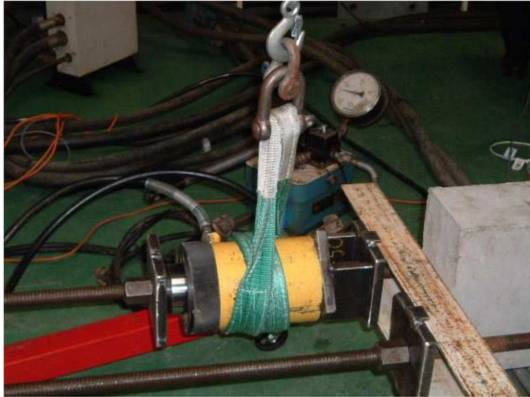
**Figure 4.11:** Stressing of Rods
