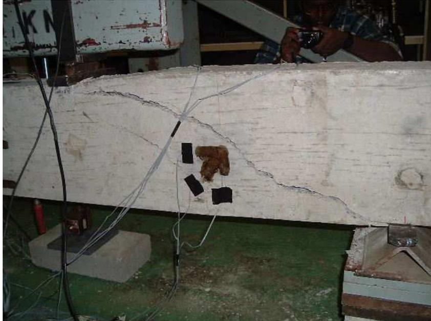
**Figure 5.2:** Failure Crack in Specimen B1
