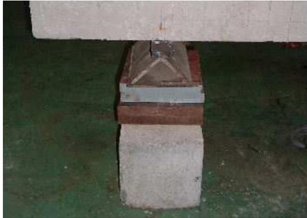
**Figure 4.14:** Test Beam Supports
