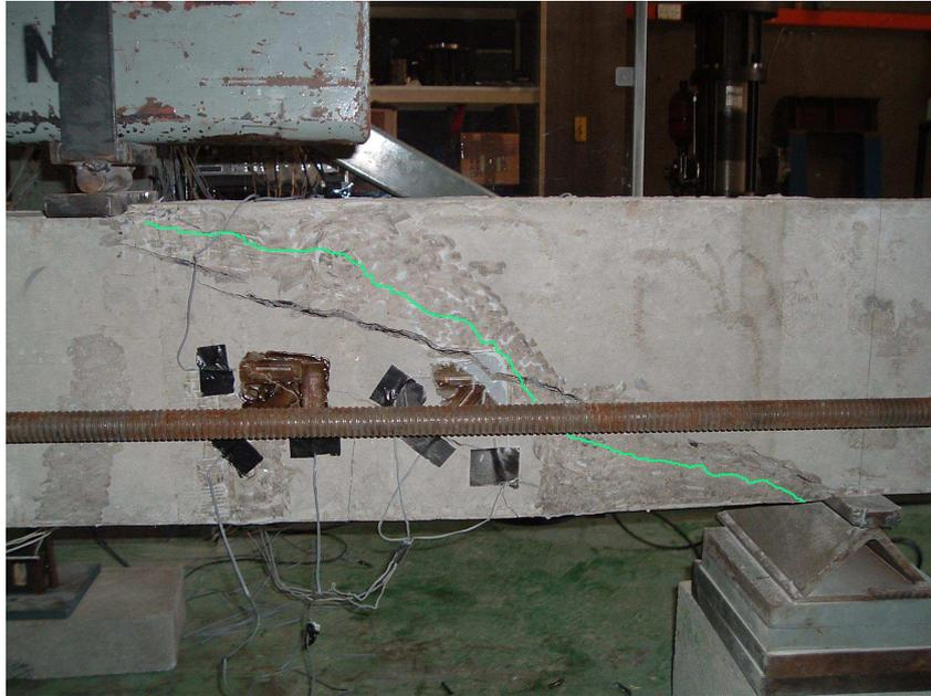
**Figure 5.6:** Failure Crack in Specimen B3
