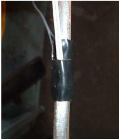
**Figure 4.5:** Steel Strain Gauge
