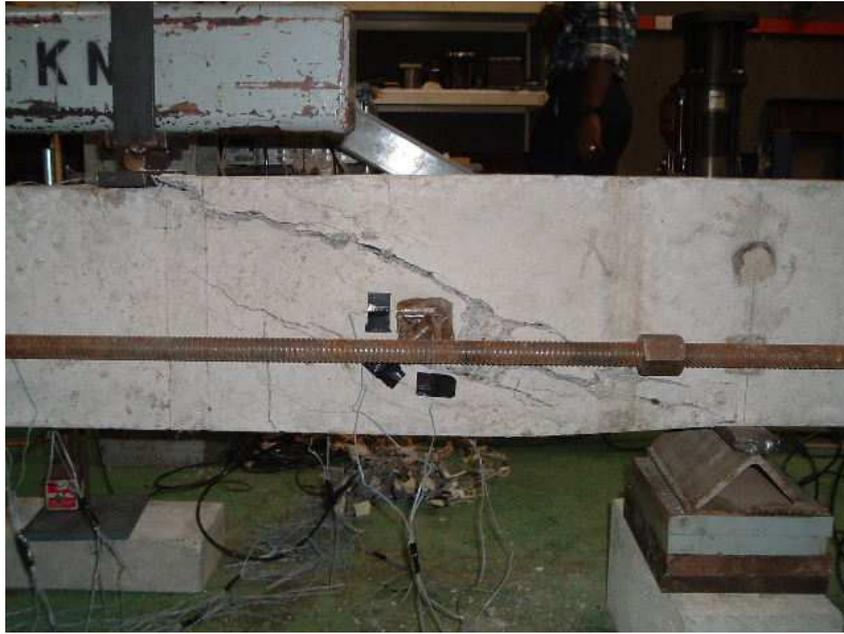
**Figure 5.7:** Failure Crack in Specimen B4
