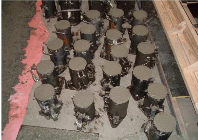
**Figure 4.7:** Freshly Cast Concrete Test Cylinders
