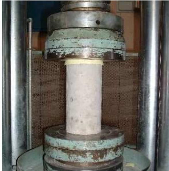
**Figure 5.1:** Cylinder Compression Test
