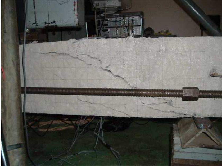
**Figure 5.4:** Failure Crack in Specimen B2
