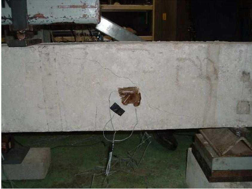
**Figure 5.5:** Initial Crack in Specimen B3
