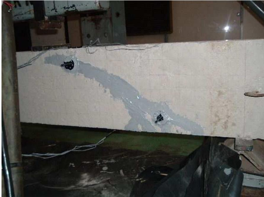
**Figure 4.12:** Sealing of Cracks Using Lokfix E
