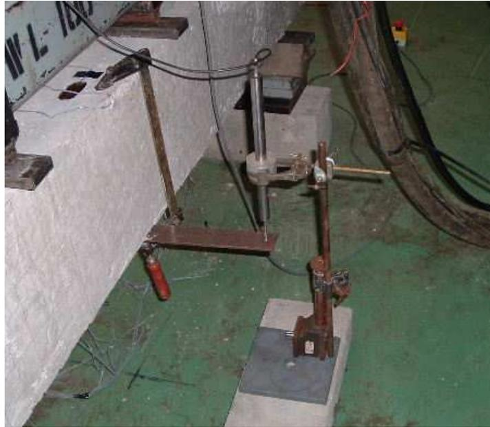
**Figure 4.15:** LVDT Measuring Midspan Deflection
