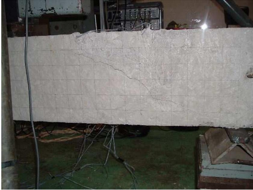
**Figure 5.3:** Initial Crack in Specimen B2
