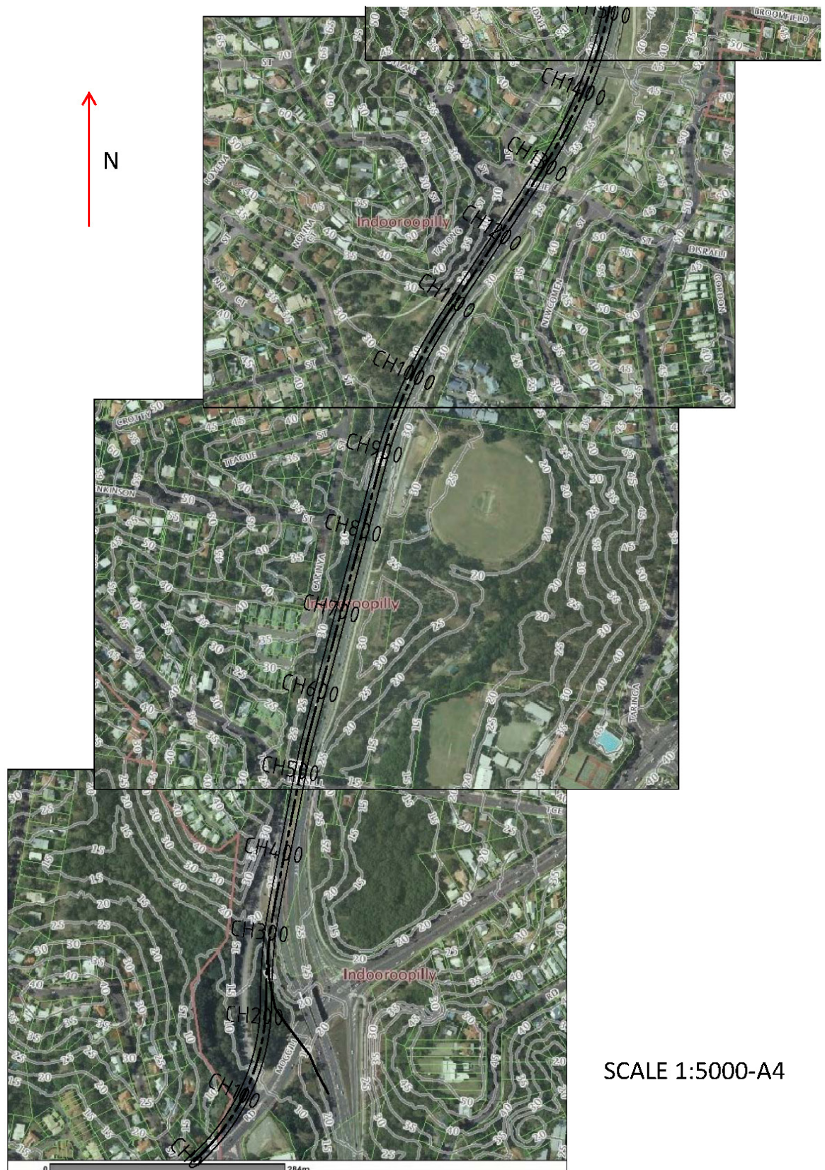
Figure 19: Proposed Elevated Western Freeway Alignment CH 0-1400
