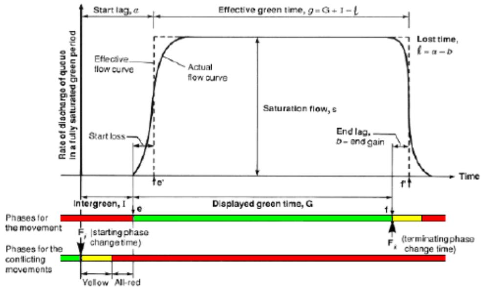
Figure 2.6: Traffic Signal Capacity
