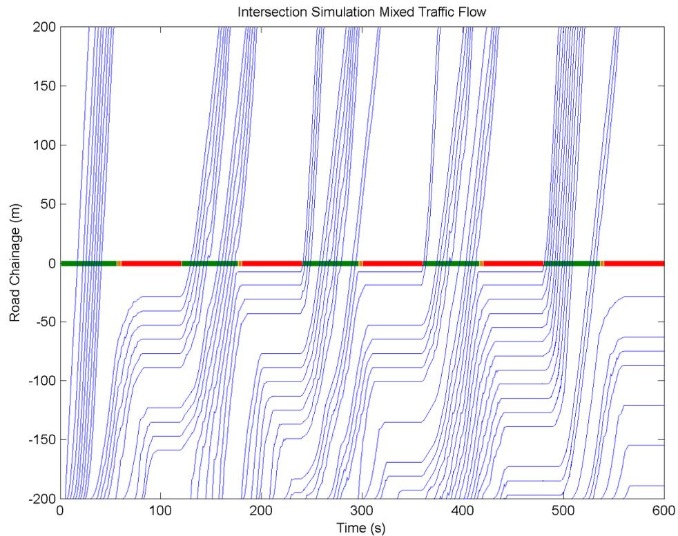
Figure 3.11: Simulation Output of Vehicle Position
