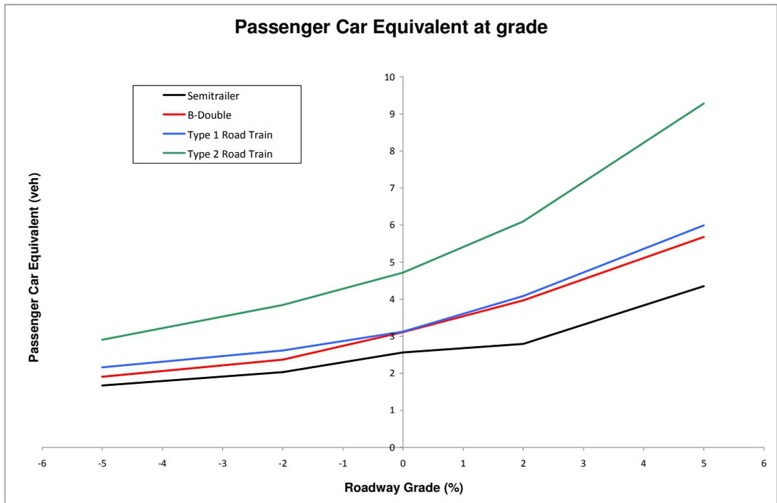
Figure 4.2: Impact of Grade on Passenger Car Equivalent Values
