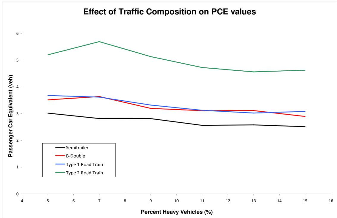
Figure 4.4: Impact of Traffic Composition on Passenger Car Equivalent Values
