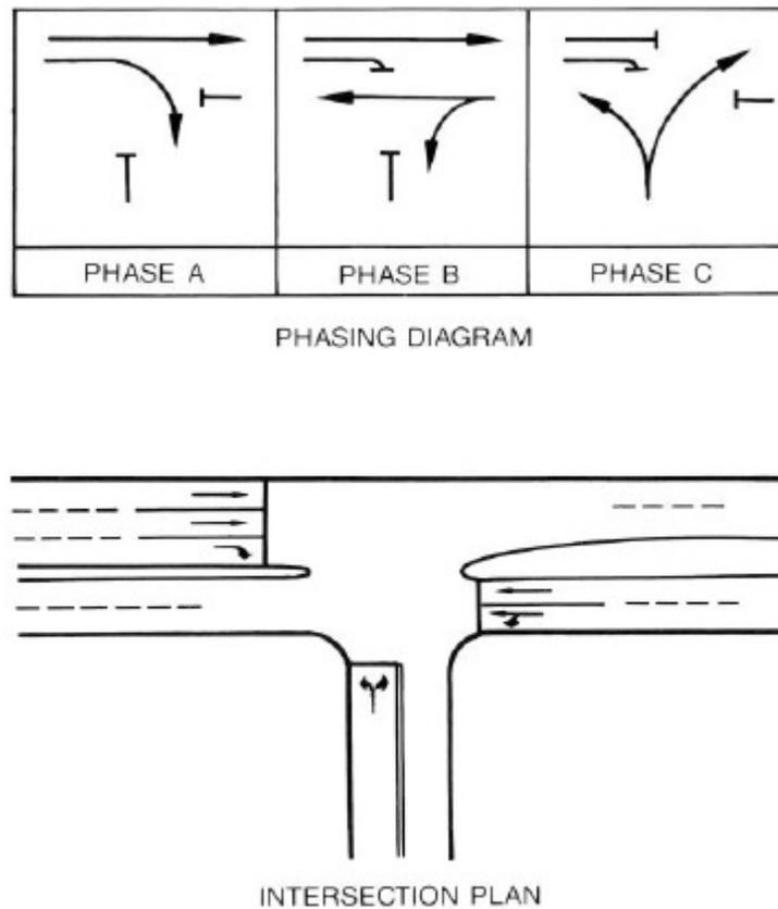
Figure 2.4: Traffic Signal Phasing Diagram
