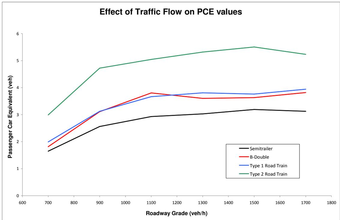
Figure 4.3: Impact of Traffic Volume on Passenger Car Equivalent Values
