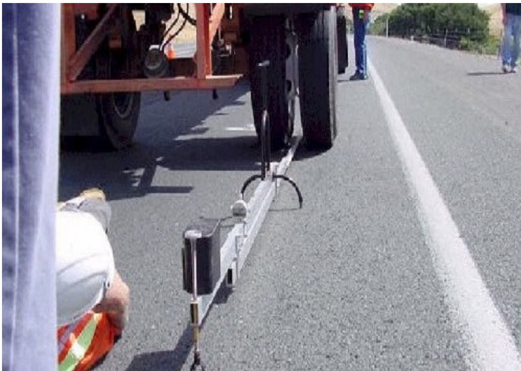
Figure 3.6 – Benkelman Beam: a) A schematic of a typical apparatus b) In use
