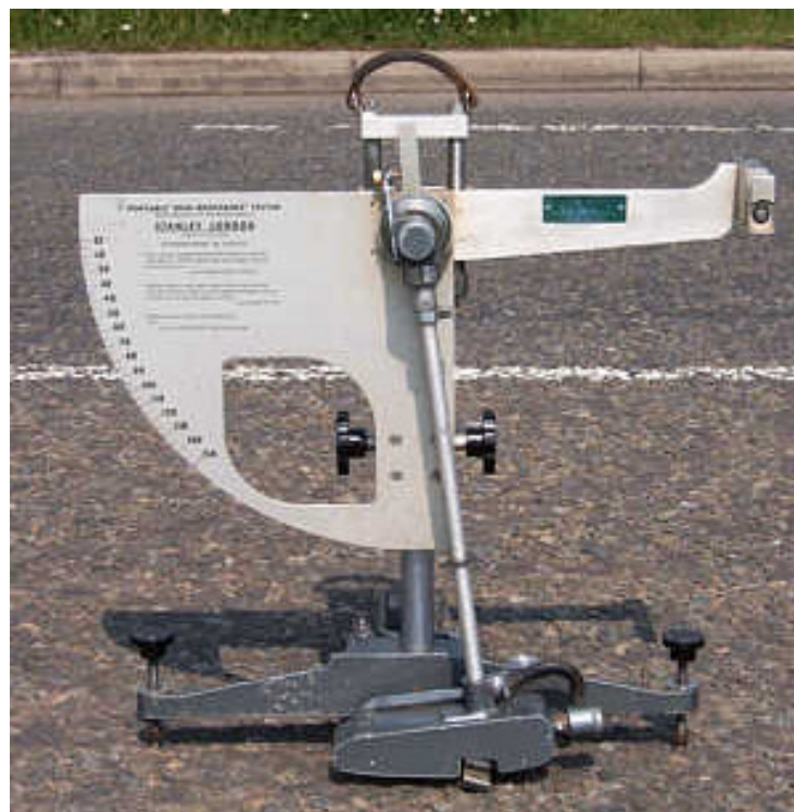
Figure 3.10 – A portable skid resistance (pendulum) tester, used for assessing skid resistance of a road surface, usually only over a small area
