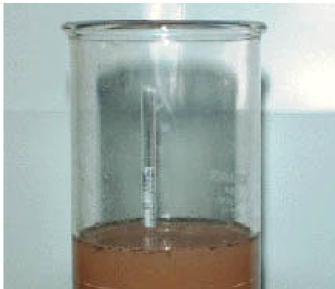
Figure 3.19 – Assessing the grading of fine particles using a hydrometer
