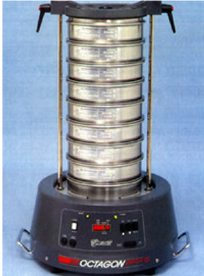
Figure 3.18 – Sieves attached to a shaker that speeds up the grading test process
