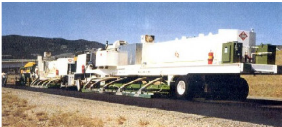
Figure 3.32 - A view of the equipment train used for hot-in-place asphalt recycling
