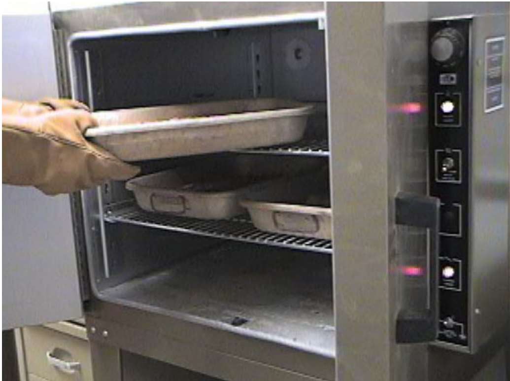
Figure 3.16 – Soil samples being put in an oven, as part of moisture content testing
