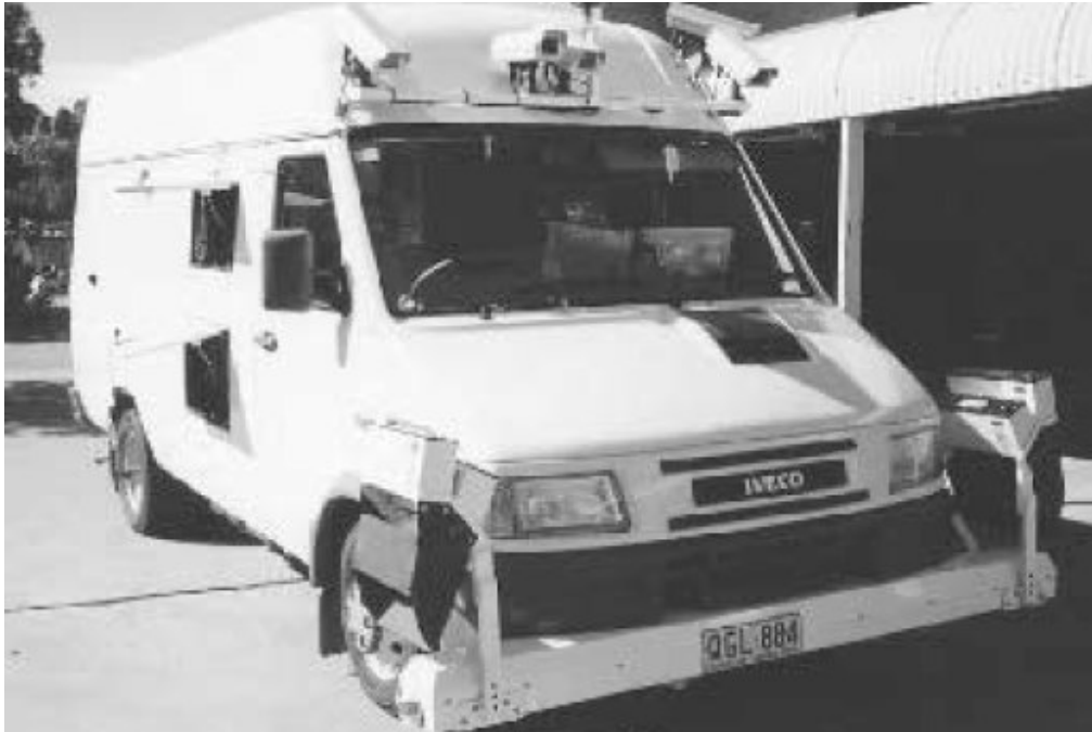
Figure 3.9 – A Network Survey Vehicle used to assess pavement properties such as roughness and rutting at the network level
