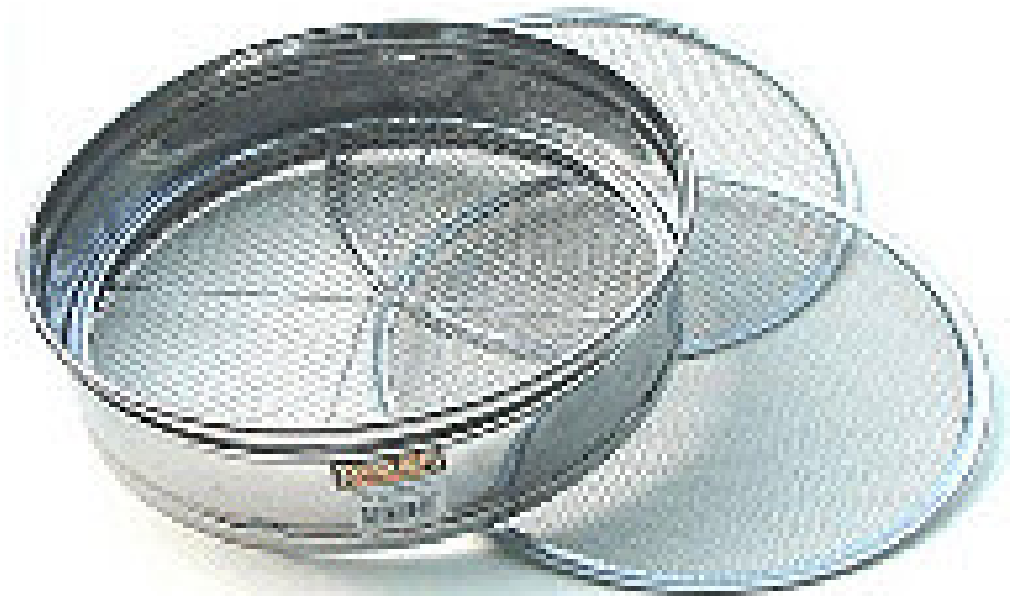
Figure 3.17 – Sieves as used to measure the particle size distribution of a soil sample
