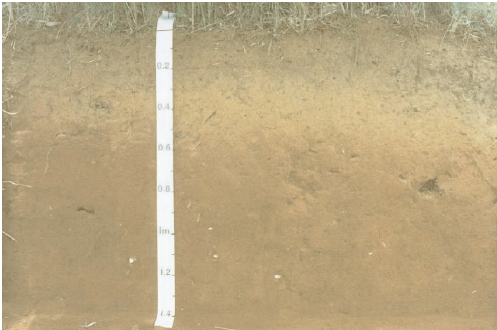
Figure 3.3 – Typical soil profiles: a) A uniform sand or sandy loam soil b) A sandy gradational soil
