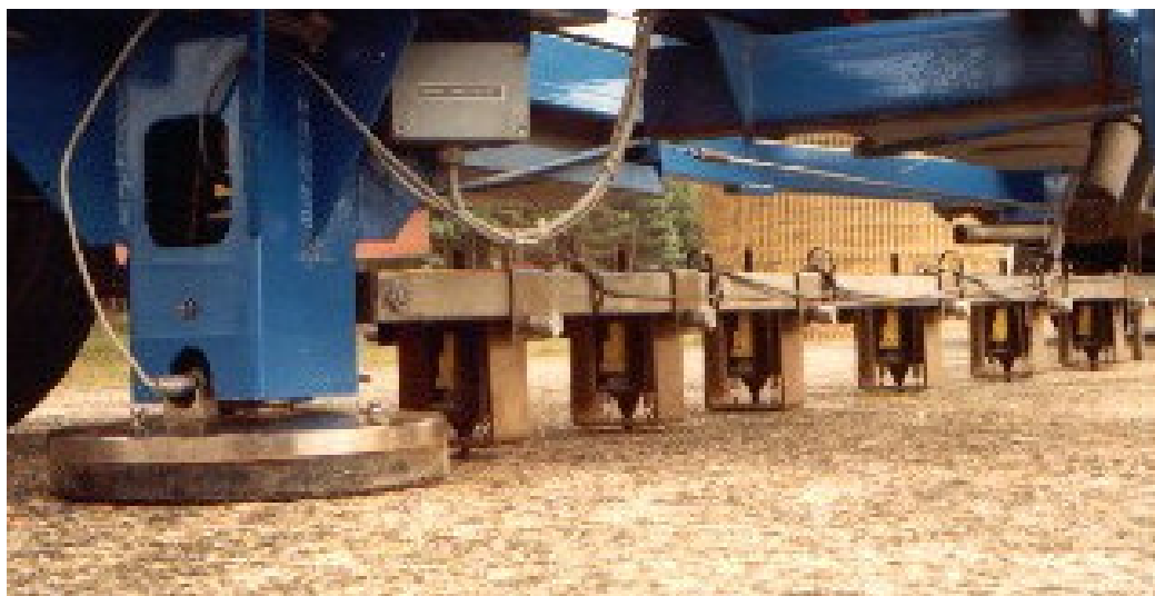
Figure 3.7 – The Falling Weight Deflectometer (FWD):
