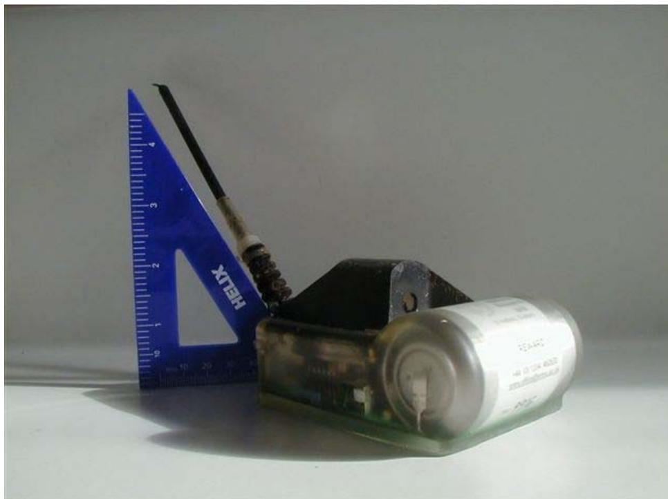
**Figure 3** The Series 7000 SLTDR uses the Argos satellite system to relay data from a surfaced seal and provides researchers with close to real time geographical positioning via a secure web address generated at the Sea Mammal Research Unit at the University of St Andrews, Scotland. Time, depth and velocity is also recorded on board and downloaded when the unit is recovered.
