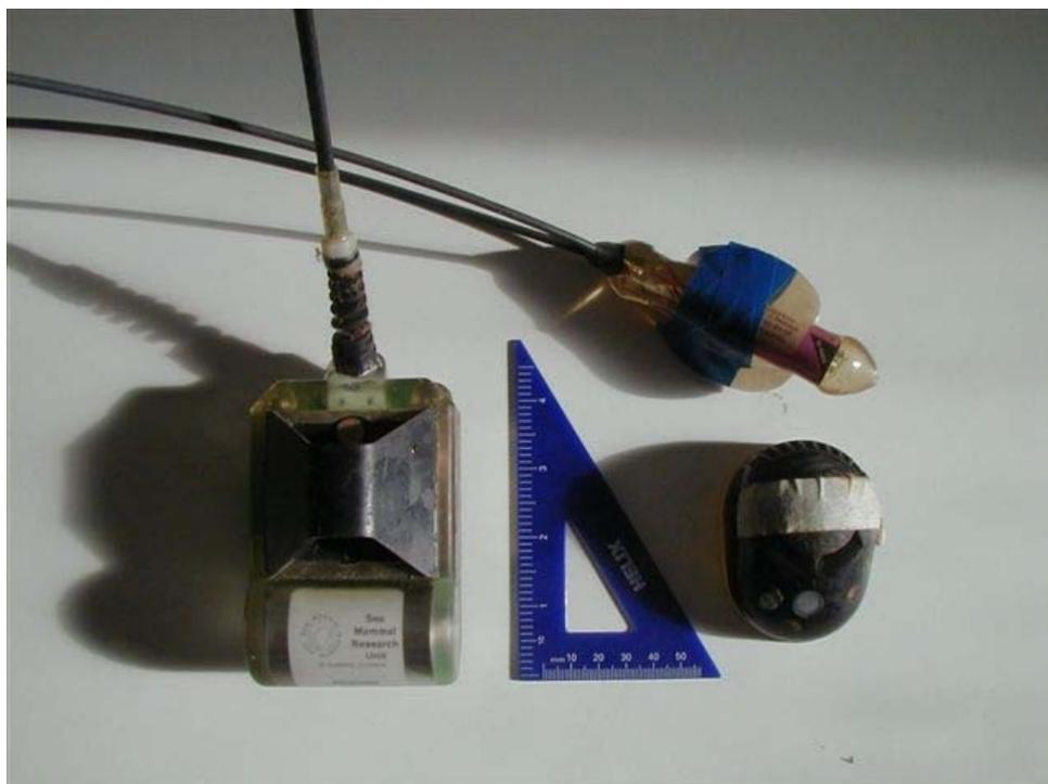
**Figure 4** SLTDR (L), VTDR (R) and VHF locator beacon (top R). The scientific payloads attached to seals are small in comparison to the target animal, an adult cow being in the order of 300kg and 2.5m in length.
