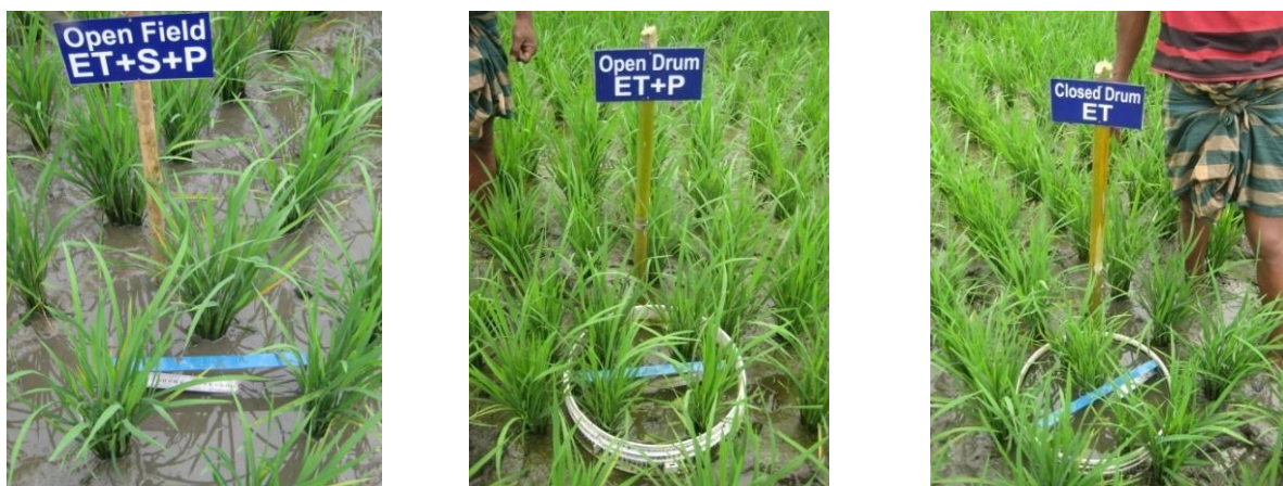
Fig. 2.5 Evapotranspiration, and percolation rate measurement by using tank and slopping gauge
