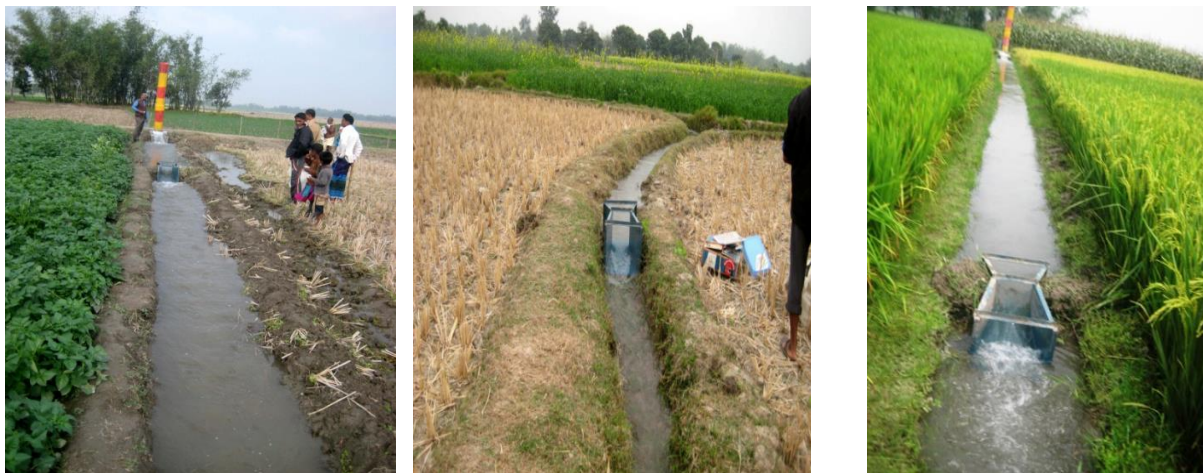
Fig. 2.4 Measurement of DTW discharge by cut-throat flume.
