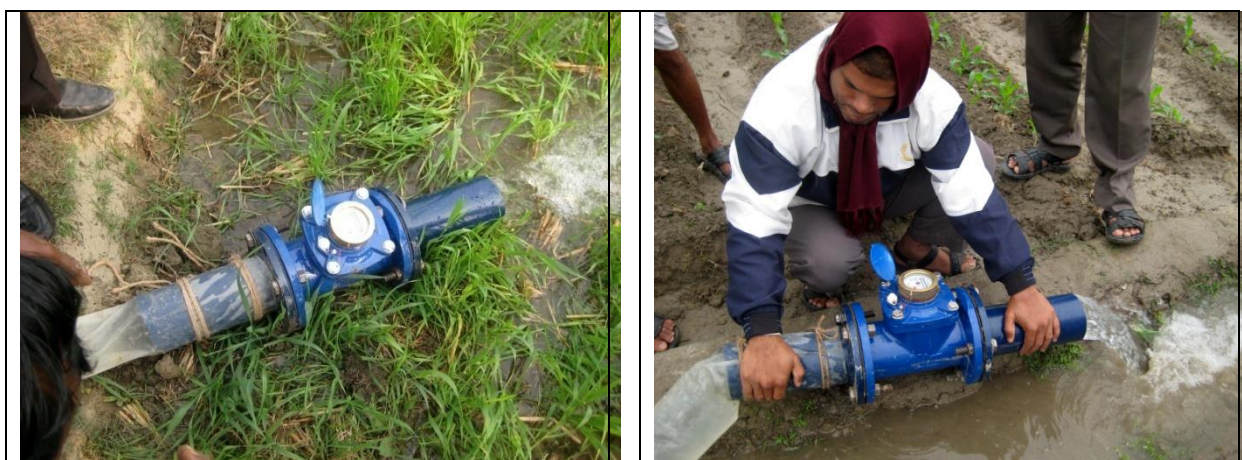
Fig. 2.3 Measurement of STW discharge by flow meter.
