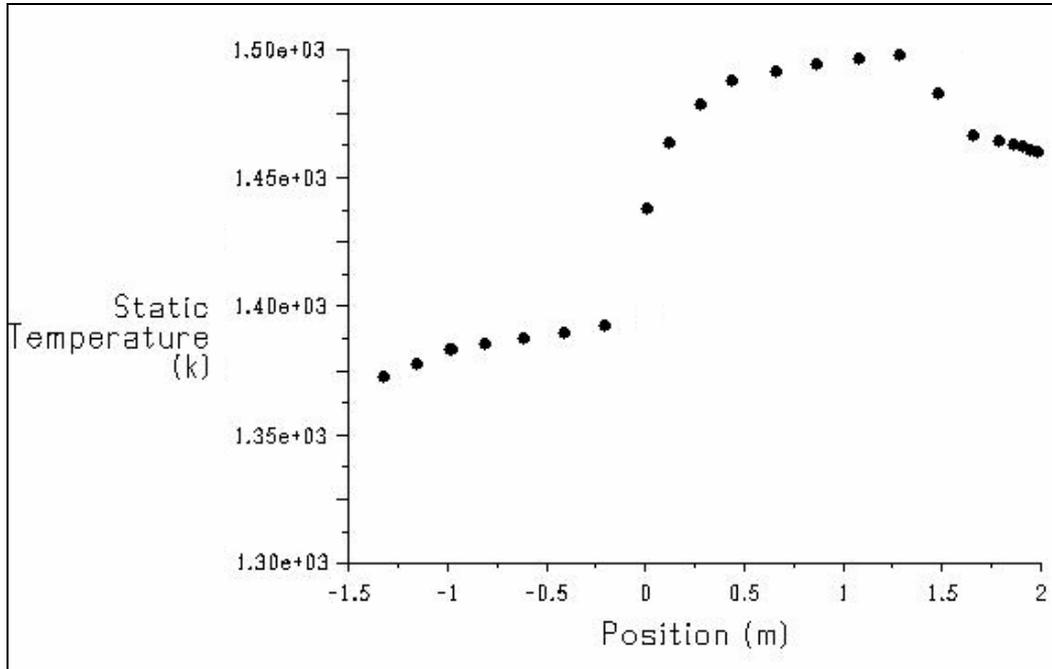
Temperature Distribution Graph for Tuyere Burner, Lid-on. 1200°C heating results from Fluent
