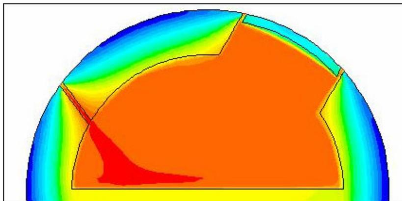
Figure 7.2: Temperature distribution for tuyere position lid-on
