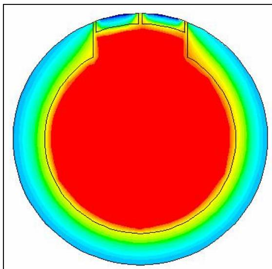
Figure 7.9: Heat distribution throughout the vessel during cold start-up
