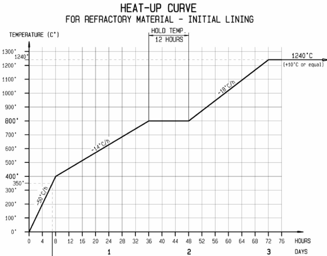
Figure 6.6: Anode furnace heat-up curve.
