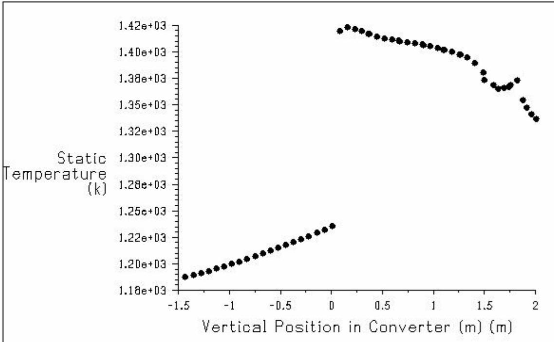
Temperature Distribution Graph for Side Wall Burner, Lid-off. 1300°C heating results from Fluent
