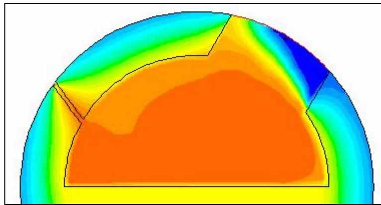
Figure 7.1: Temperature distribution for tuyere position lid-off
