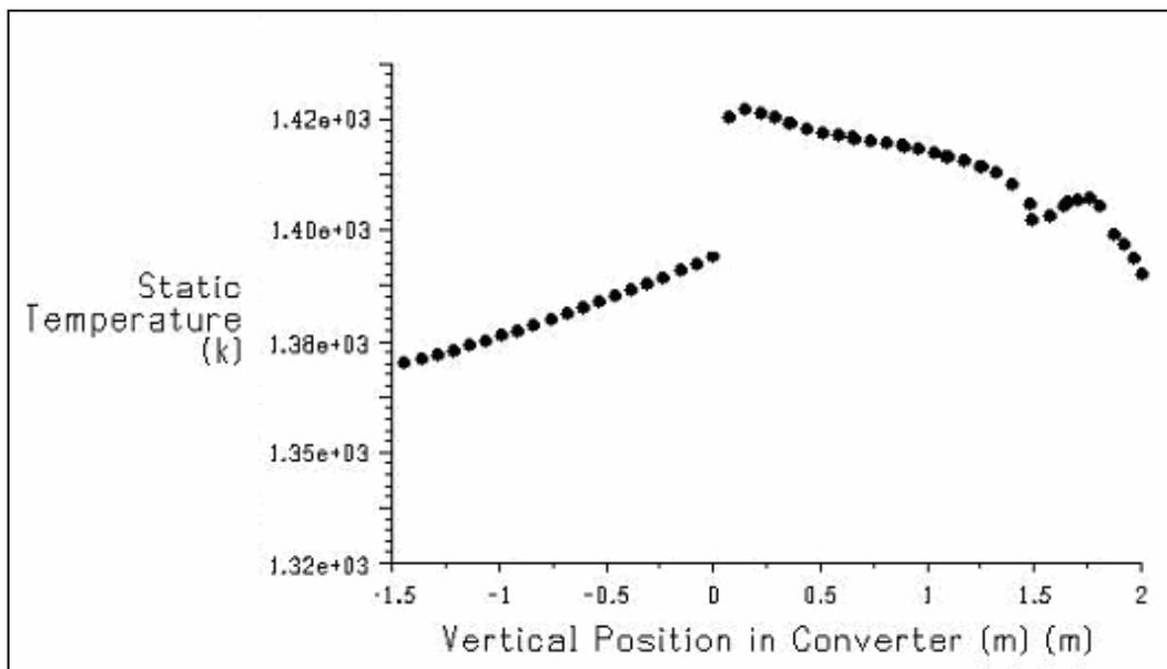
Temperature Distribution Graph for Side Wall Burner, Lid-on 1200°C heating results from Fluent
