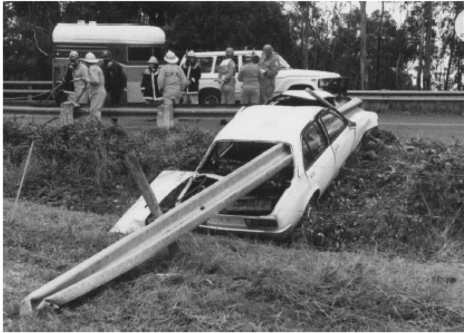
Figure 2.4 Guardrail speared through passenger compartment of vehicle. Hayworth 1997 in Grzebieta & Reznitz (2001a)
