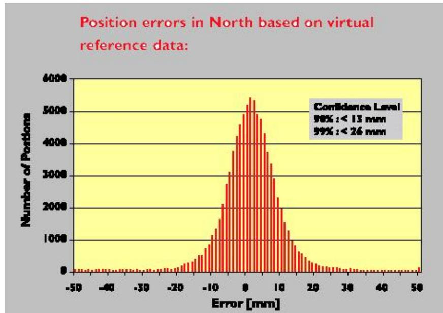
Figure 2.3: The expected Horizontal accuracies of GPSnet.dk (*The idea behind GPSnet.dk is simple - VRS is ingenious* 2005)
