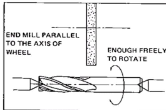
Fig.38. Holding End mill
