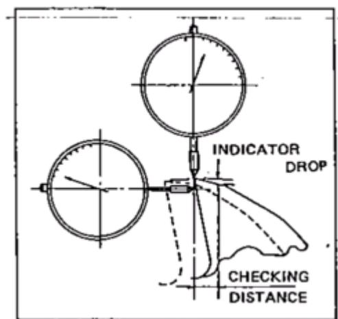
Fig.56. Indicator Set-Up for checking Radial Relief
