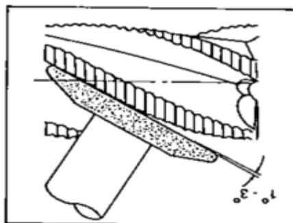
Fig.50. Angle of Wheel Inclination
