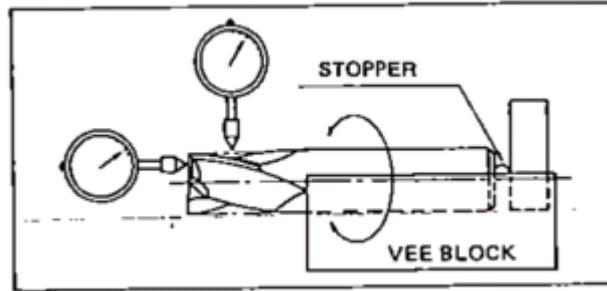
Fig.58. Measuring Cutter Run-outs
