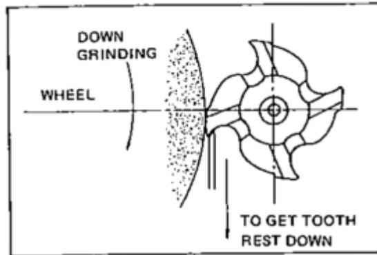
Fig.47. Grinding Secondary Clearance
