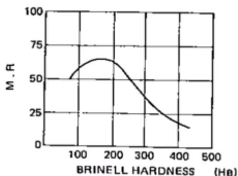
Fig.27. Relation between M.R and hardness of Steel
