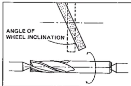
Fig.41. Wheel Inclination
