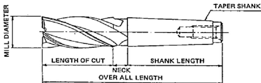
Fig.2. Taper Shank End mill
