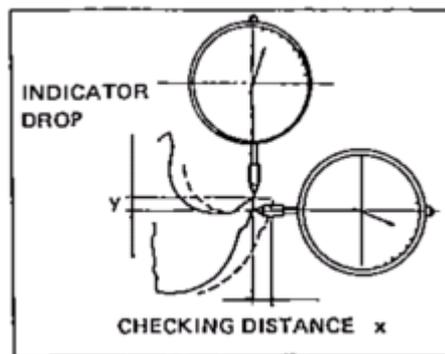
Fig.57. Checking Cutting Angle
