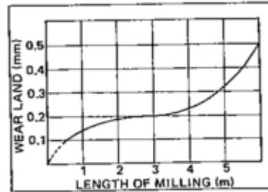
Fig.34. Relation between Wear Land & Length of Milling
