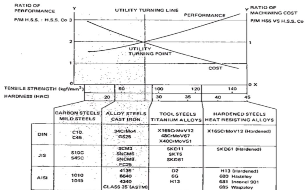
Fig.18. Performance vs. Machining Cost
