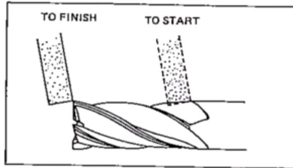
Fig.43. Trial Grinding
