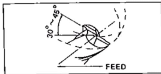
Fig.55. Re-Sharpening Gash
