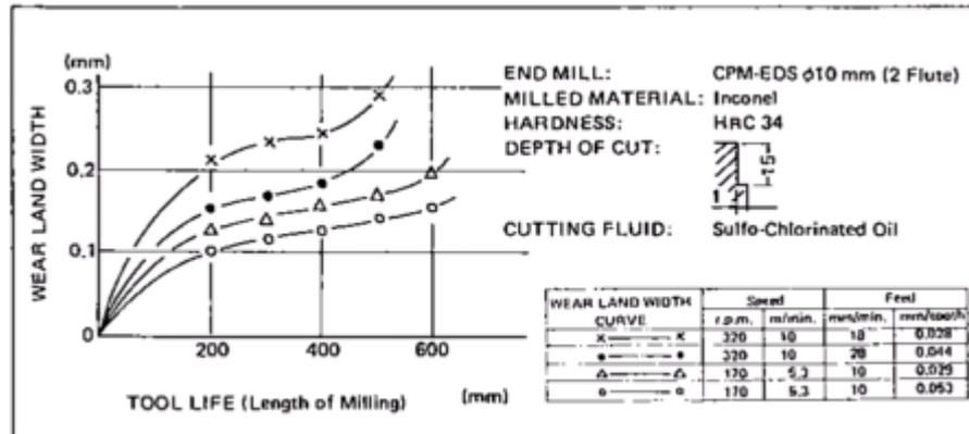
Fig.29. Milling test on Inconel material
