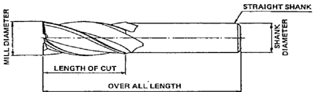
Fig.1. Straight Shank End mill
