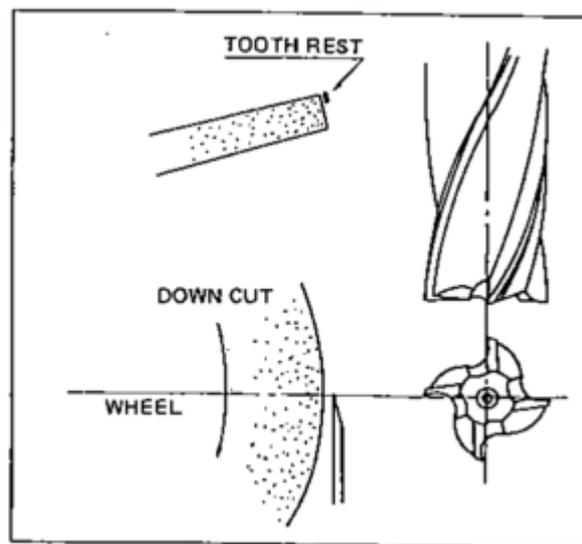
Fig.42. Position of wheel, End mill and tooth rest
