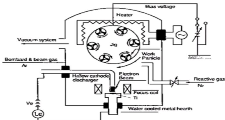
Fig.25. Physical Vapor Deposition Process
