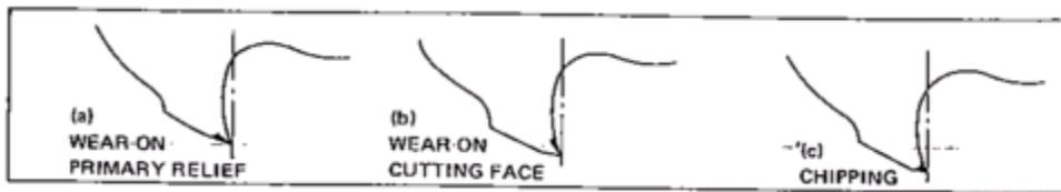
Fig .32. Damages of Cutting Edge
