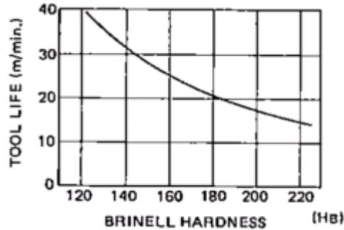
Fig.28. Relation between Tool life and Work hardness
