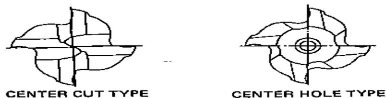
Fig.7. Different type of Cutting Edge
