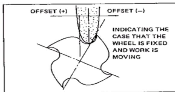
Fig.51. Adjustment of Offset
