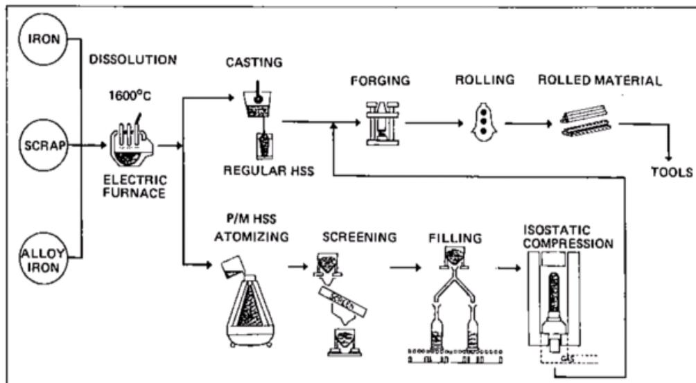
Fig.16. Manufacturing Process: Particle Metallurgy H.S.S. vs. Regular H.S.S.
