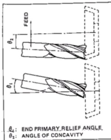
Fig.53. Grinding of End Primary Relief
