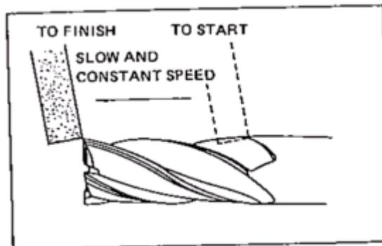
Fig.45. Grinding Primary Relief
