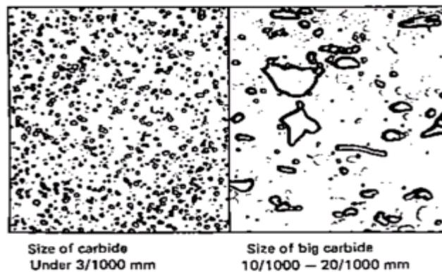
Fig.17. Microscope Photograph (Magnification: X400)
