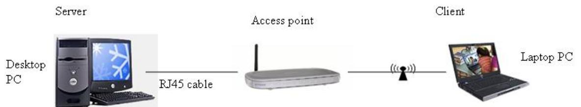
Figure 5.7: Experimental setup.
