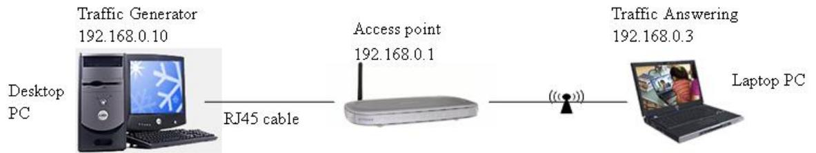
Figure 6.3: WLAN configuration.
