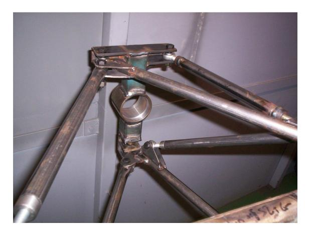
Figure 3E Rear Suspension Assembly
