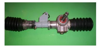
Figure 28 Modified steering box assembly
