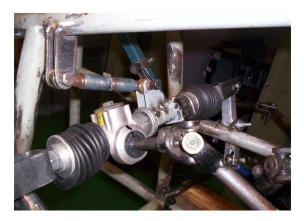
Figure 4E Steering Box Assembly on the Chassis
