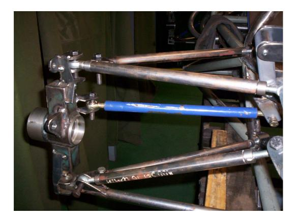
Figure 2E Front Right Suspension Assembly
