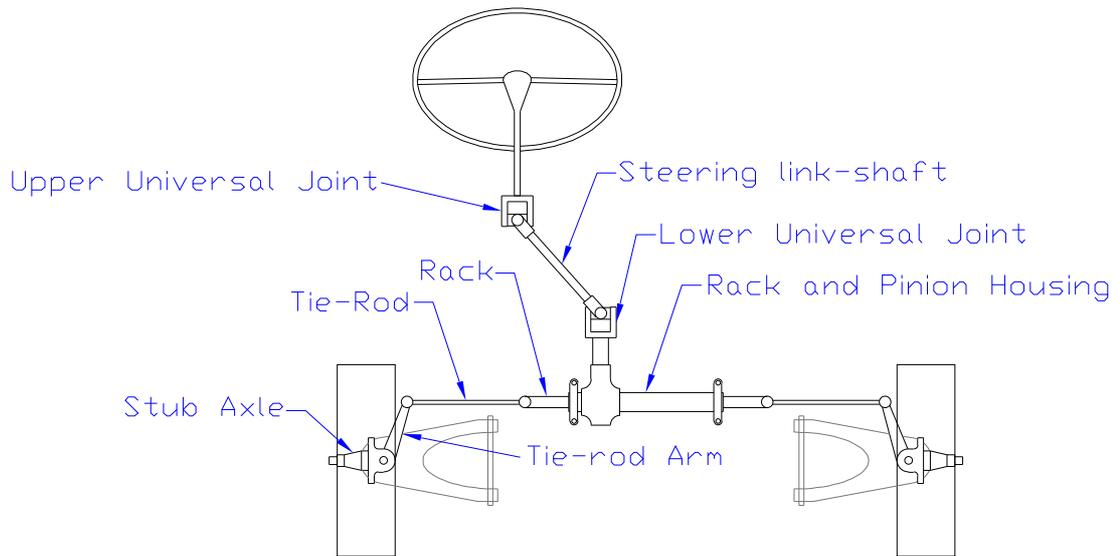
Figure 2.12: Rack and pinion steering linkage.
