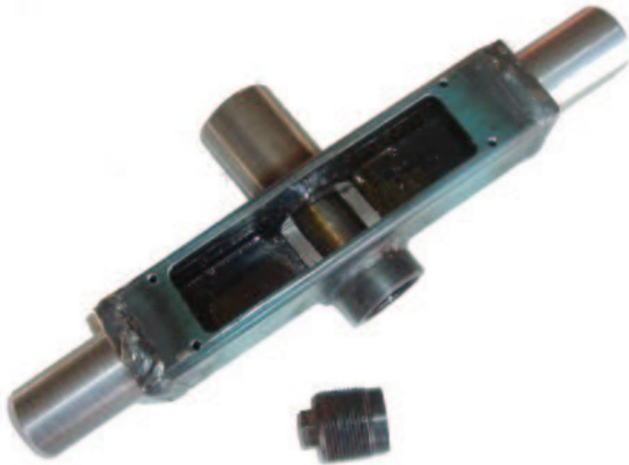
Figure 4.3: Complete housing for modified rack and pinion.
