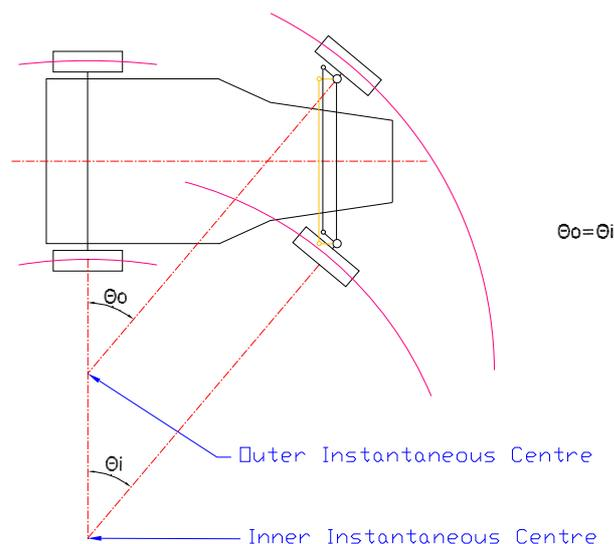
Figure 2.3: Parallel track-rod arms giving true rolling at straight ahead only.
