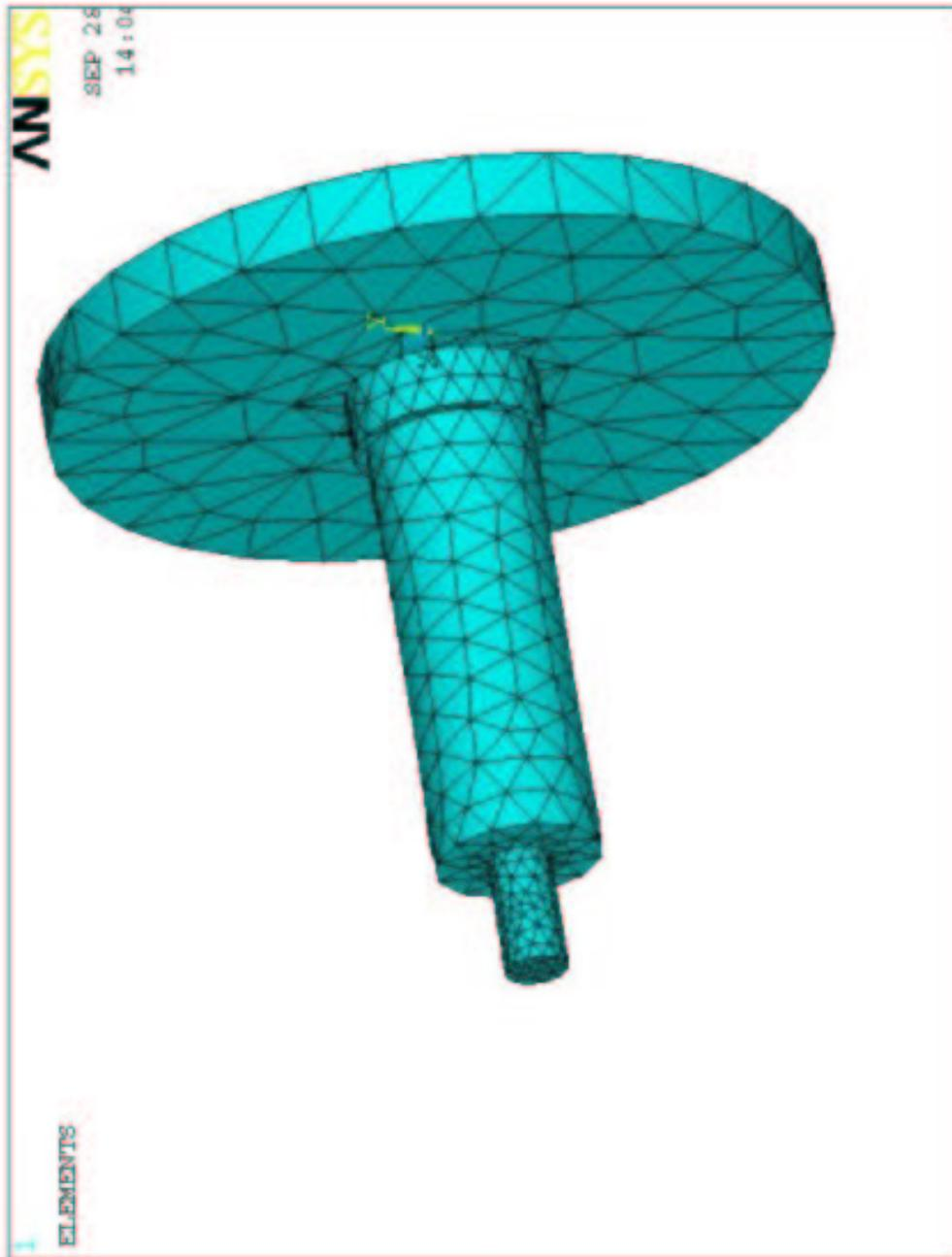
Figure D.1: Finite element mesh for axle using Ansys.
