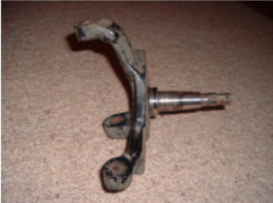
Figure 5.1: Typical motor vehicle stub axle design.
