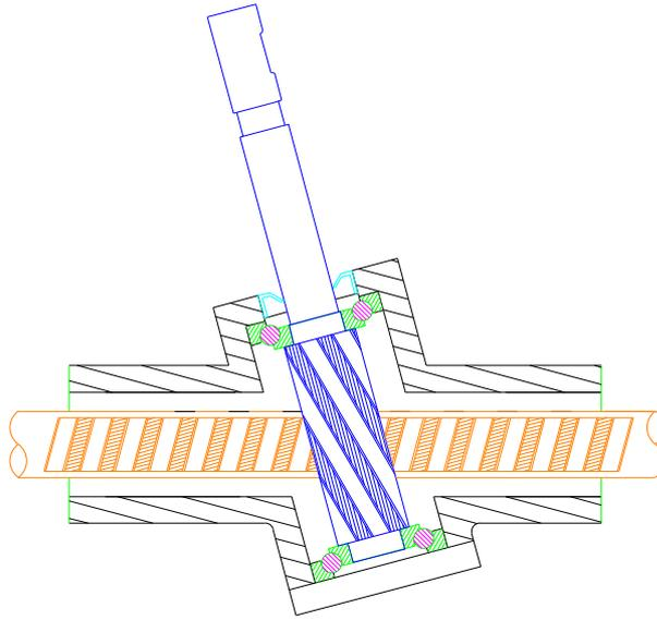
Figure 2.13: Helical rack and pinion steering gear with tilted pinion axis.
