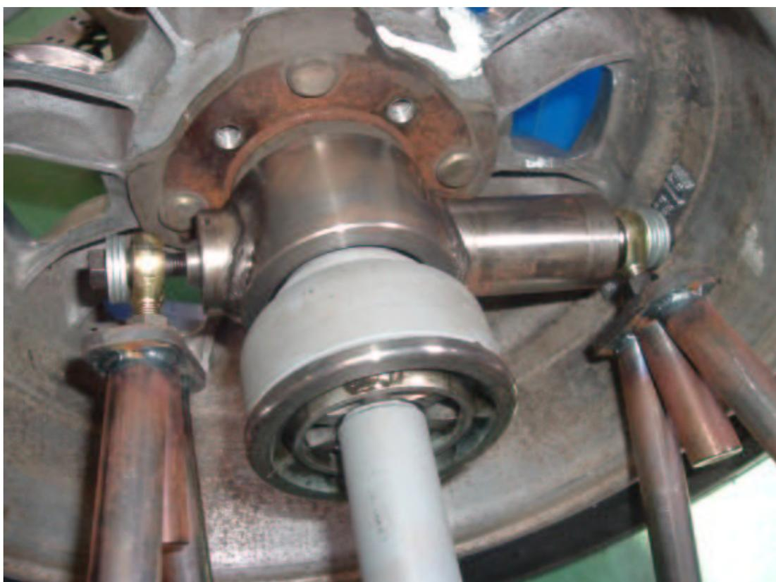
Figure B.5: Rear upright mounted in road wheel and suspension arms.
