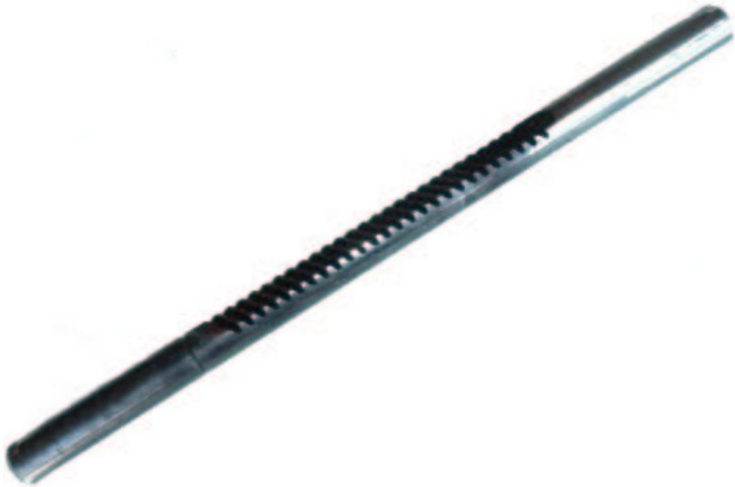
Figure 4.2: Renault R10 rack after modification.
