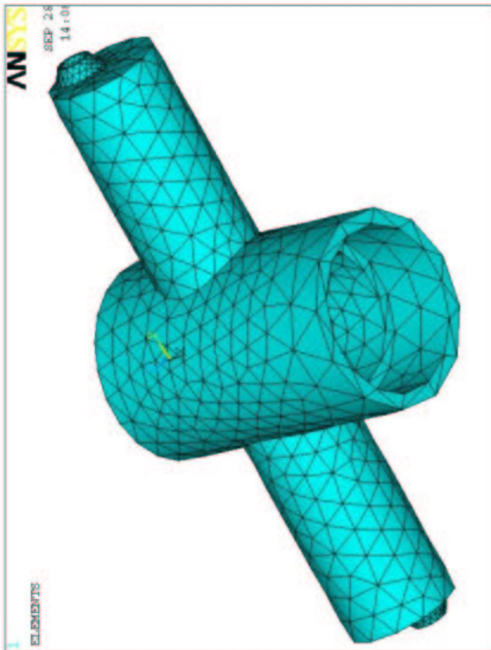
Figure C.1: Finite element mesh for upright using Ansys.
