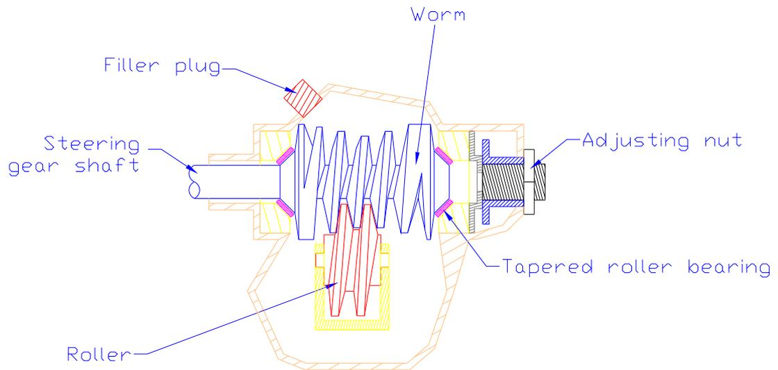
Figure 2.17: Worm and roller steering box.
