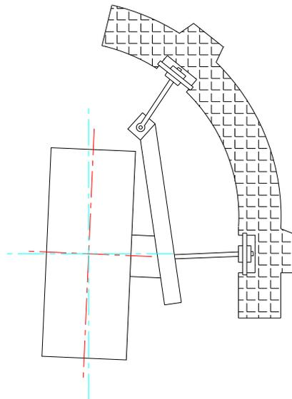
Figure 2.9: Porsche 928 system with brake drag. Note the link's deflection giving the wheel slight toe in.
