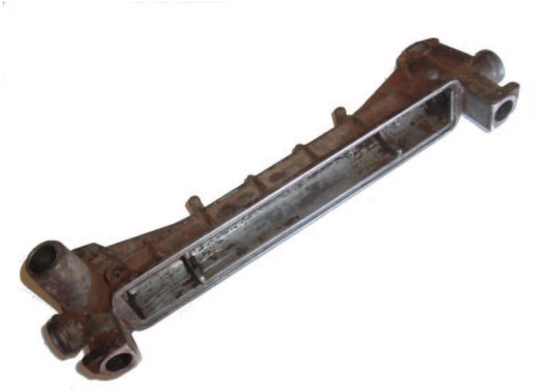
Figure 4.1: Renault R10 rack housing. Note: Pinion is offset to far left hand end of housing.
