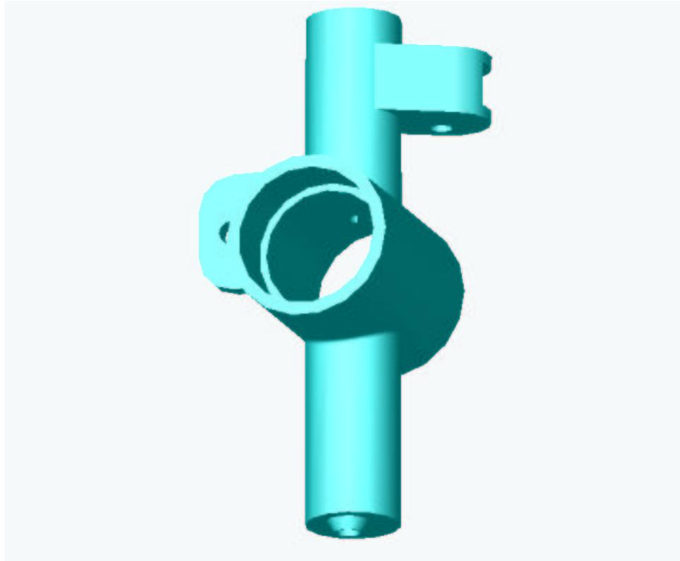
Figure 5.12: Left view of final model of left upright.
