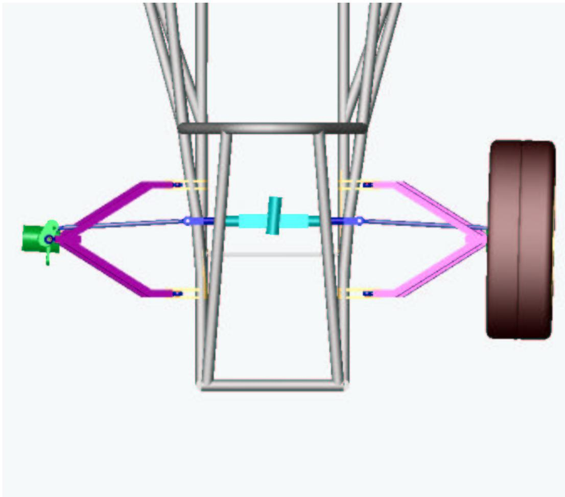
Figure 7.2: Final model of the steering system.
