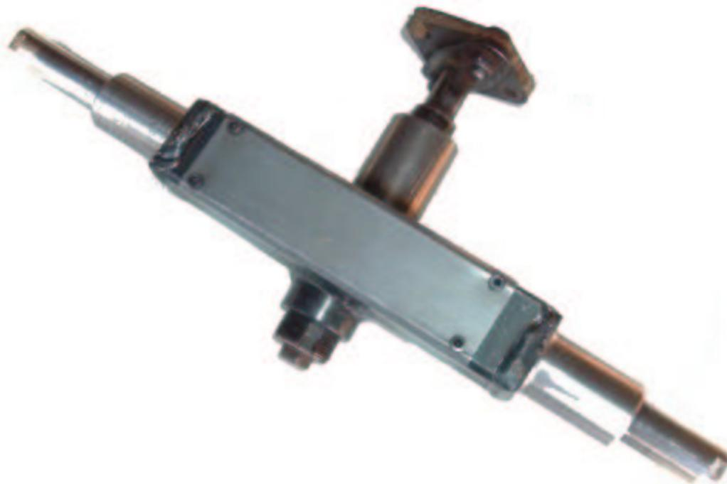
Figure B.1: Completed rack and pinion steering box.
