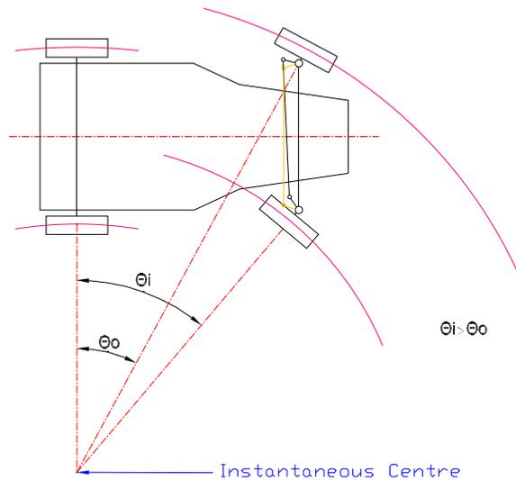
Figure 2.4: Inclined track-rod arms giving true rolling in three positions.
