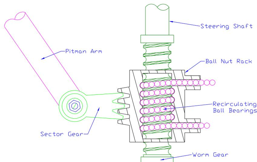
Figure 2.15: Recirculating ball steering box.
