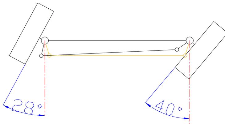
Figure 2.5: Outer wheel turns at a greater angle than the inner wheel.
