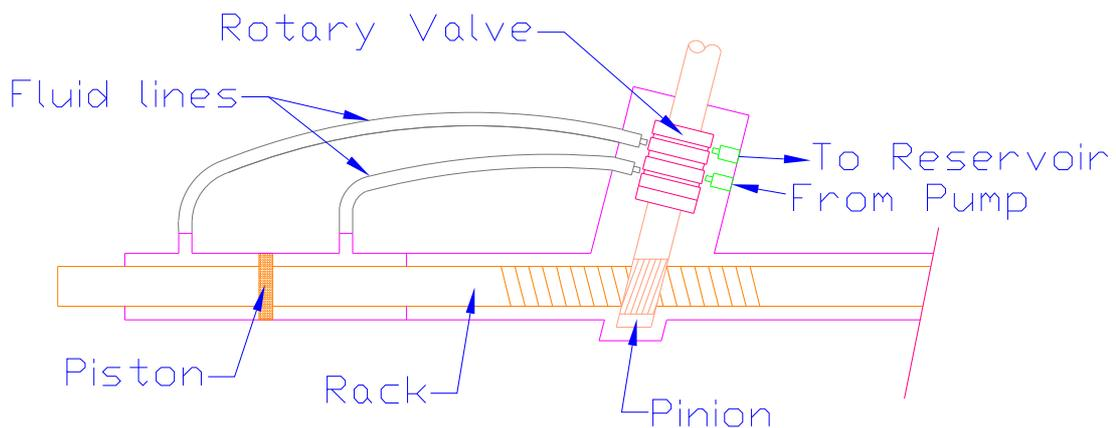
Figure 2.14: Power assisted rack and pinion steering box.
