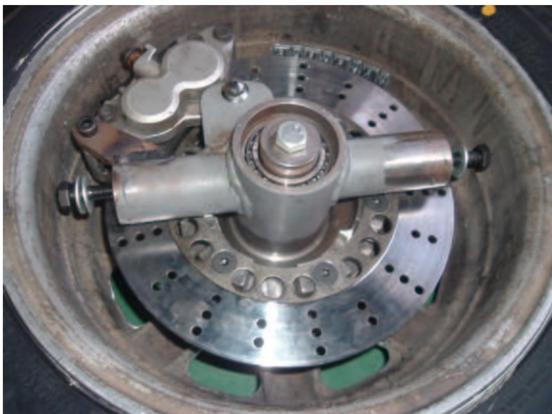
Figure B.3: Front upright mounted in road wheel.
