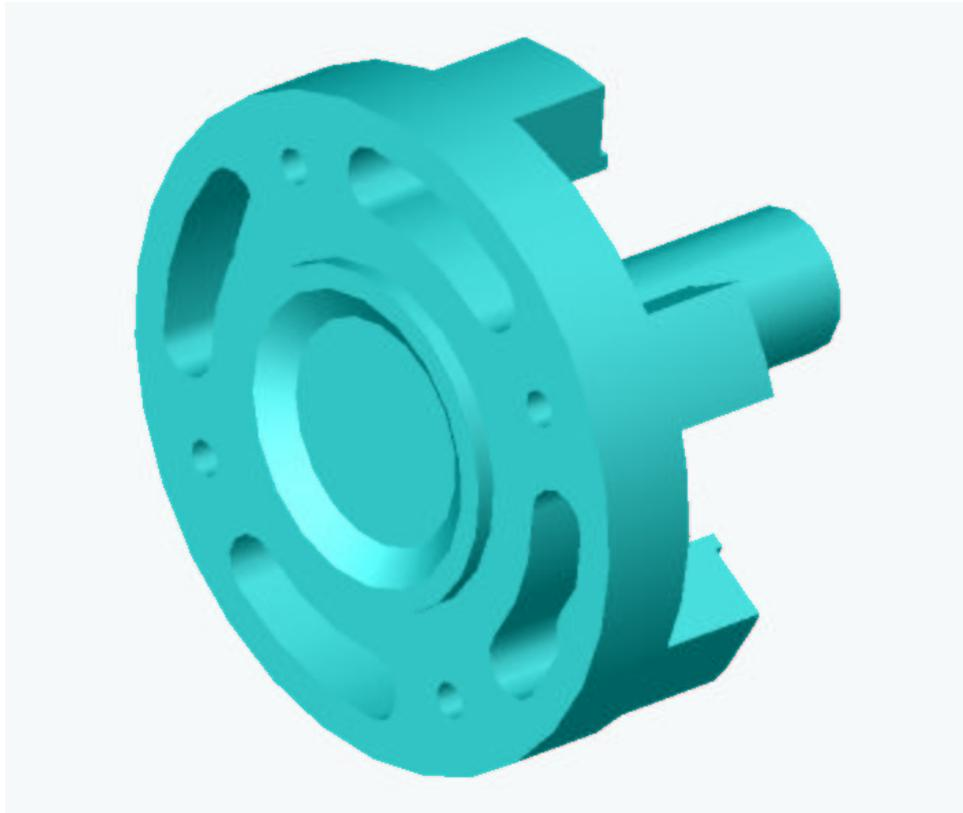
Figure 5.9: Isometric front view of final model of axle.
