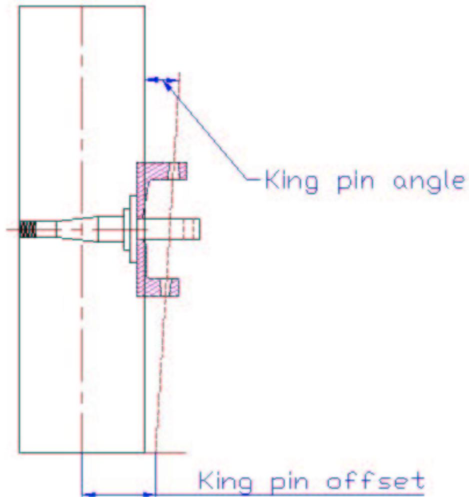
Figure 3.1: King pin angle and offset.
