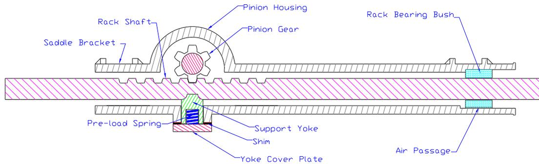
Figure 2.11: Rack and pinion steering box.
