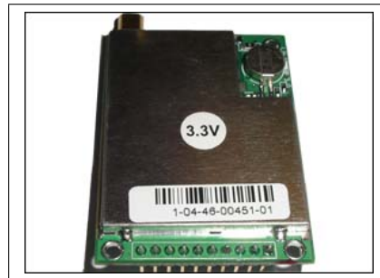
Figure E.4: LS-40EB GPS module
