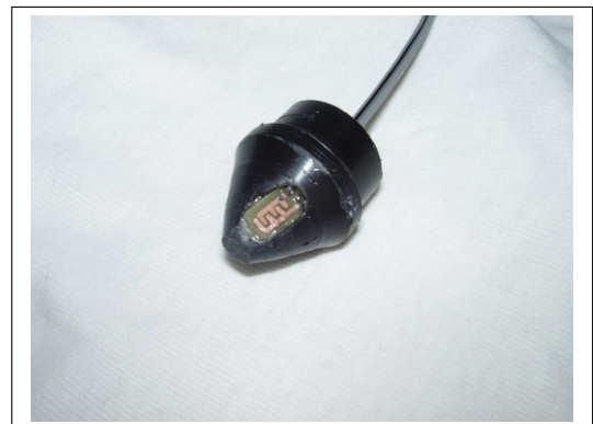
Figure 7.7: Water detector using PCB pattern
