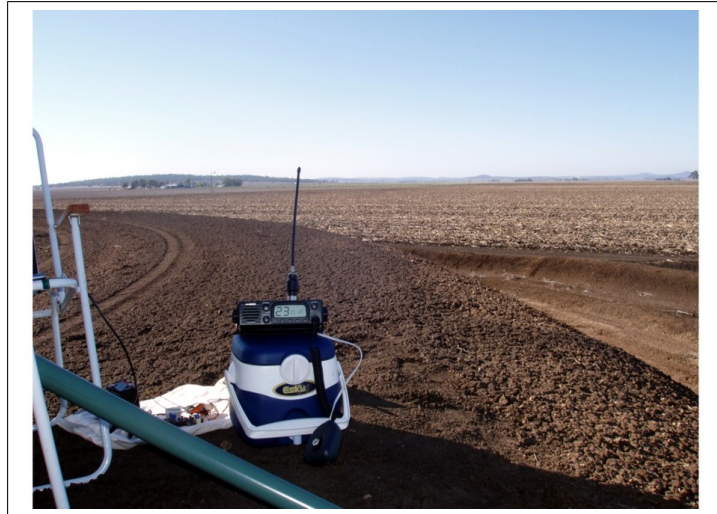
Figure 8.10: Base station with antenna mounted 4 m above fields
