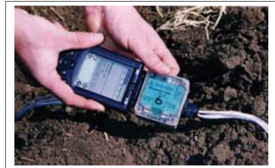
Figure 2.4: Downloading information from advance meter to PDA
