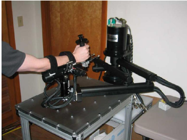
Figure 2.6: The MIT-Manus is a highly function robotic rehabilitation device with 5 DOFs to exercise the shoulder, elbow and wrist (Source: Garrett, 2009)
