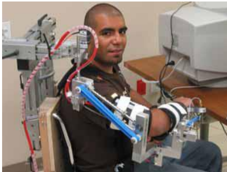
Figure 2.4: The T-WREX is an weight reducing structure that has been designed to support an arm weakened by paralysis (Source: Housman et al, 2007)
