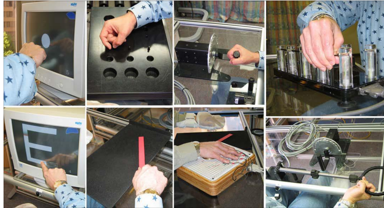
Figure 2.3: The eight tasks performed at the Auto CITE workstation are reaching, peg board, supination/pronation, threading, tracing, object-flipping, fingertapping and arc-and-rings
