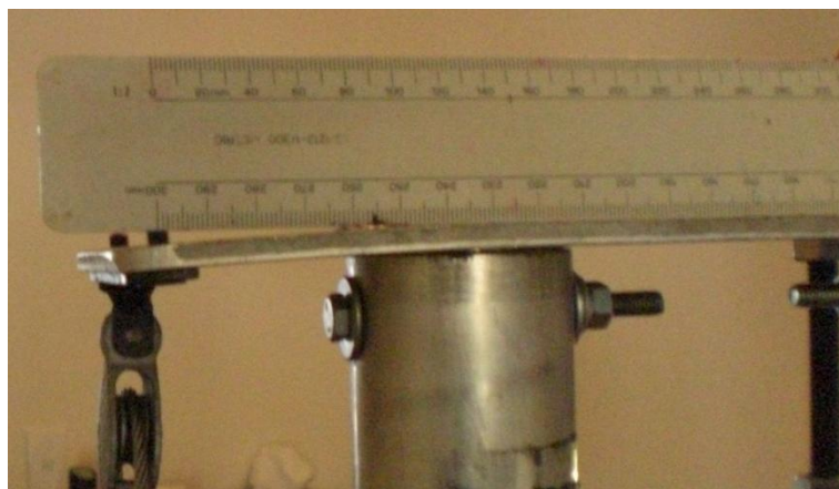
Figure 7.1: Photograph showing the bending that the top bar has experienced.
