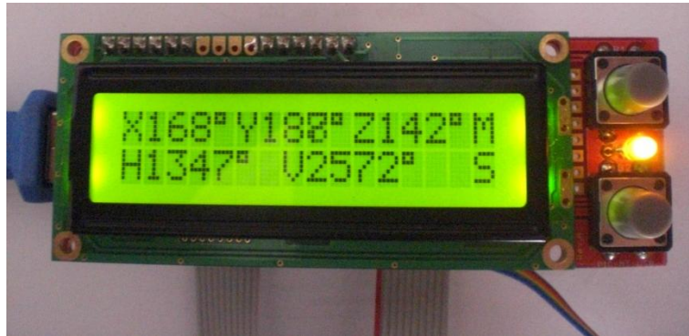
Figure 6.2: Photograph of the LCD screen in rotation mode showing the relative angel of each of the potentiometers.
