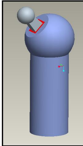
Figure 6.3 - The simplified assembly of the cemented femoral system in ProEngineer
