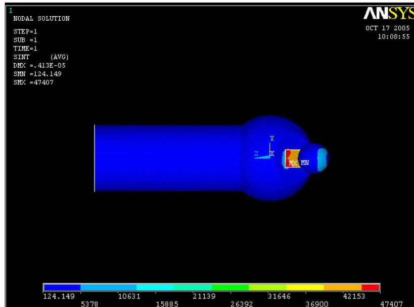
Figure 5.11 – The stress intensity in the un-cemented hip components in the x-y plane for 1 contact pair
