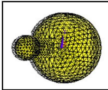
Figure 6.12 - The deformation in the x-y plane for the first analysis of the cemented hip
