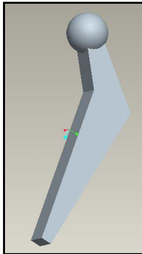
Figure 5.1 - The simplified un-cemented model of the femoral stem
