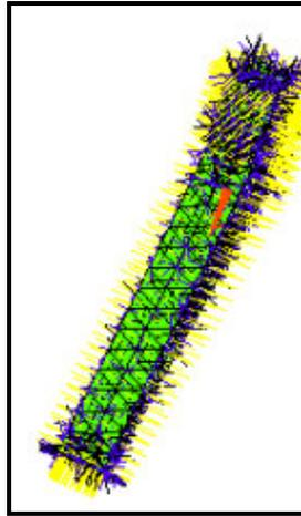
Figure 5.5 - The contact pair that was created for the bone between the bone and the implant
