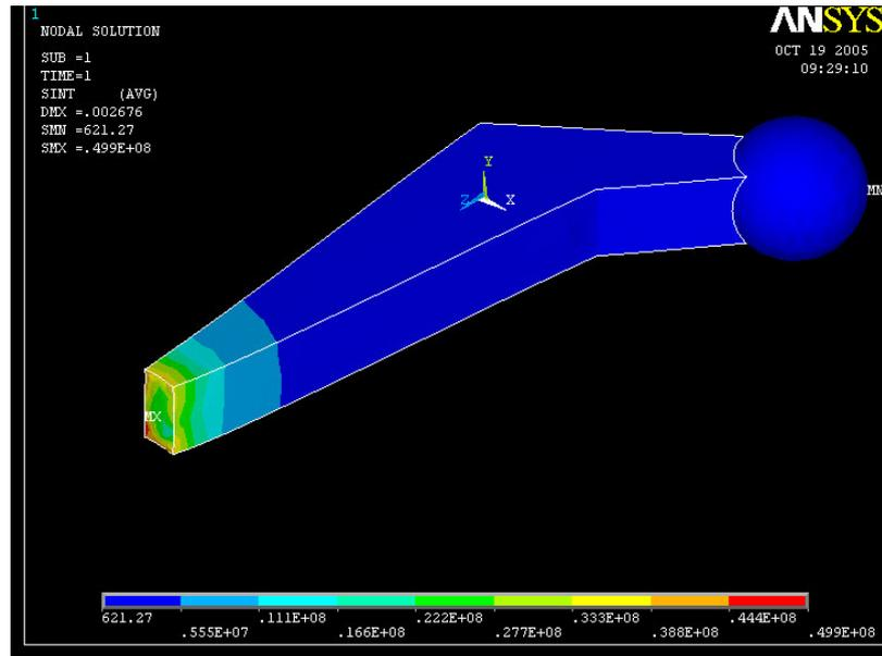
Figure 6.15 - The stress distribution of the femoral stem for the first analysis of the cemented hip
