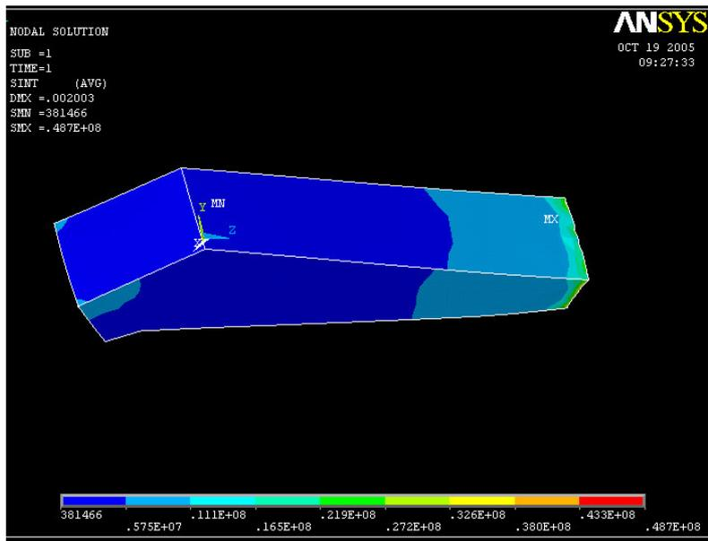
Figure 6.14 - View 2 of the stress distribution in the cement for the first cemented hip analysis
