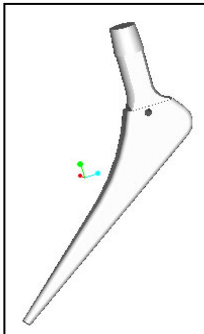
Figure 4.5 - The complete assembly of the cemented femoral stem
