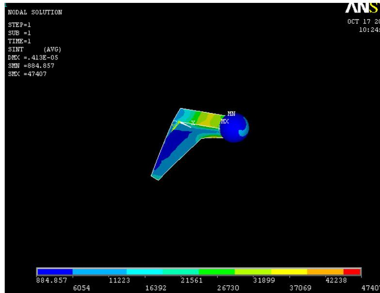
Figure 5.13 – An isometric view of the femoral stems showing the stress on the lateral side for 1 contact pair
