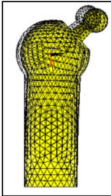
Figure 5.8 – The deformed and undeformed shape for the un-cemented FEA in the z-x plane
