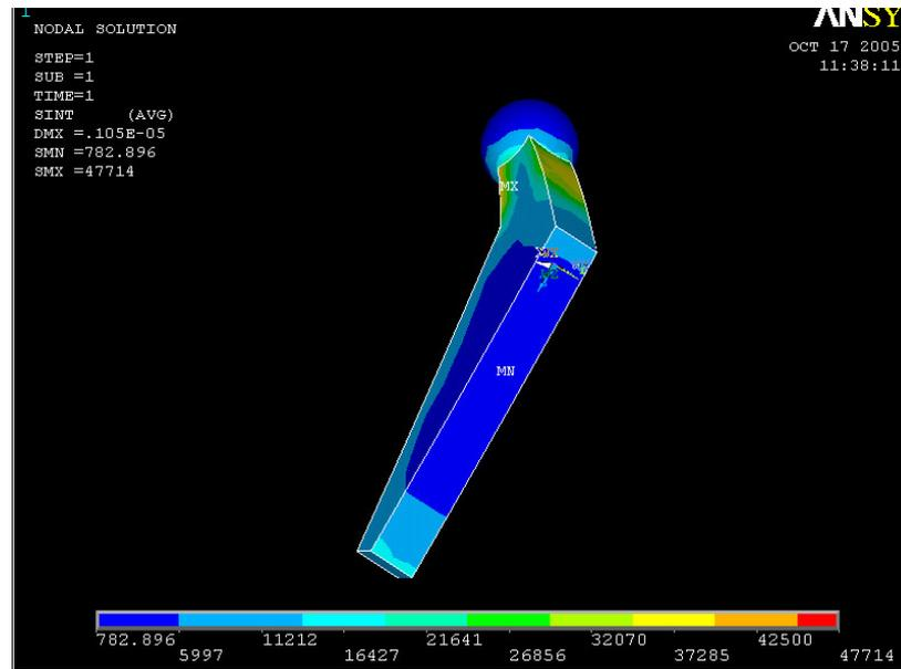
Figure 5.19 - View 2 of the stress intensity for the un-cemented femoral stem with 2 contact pairs
