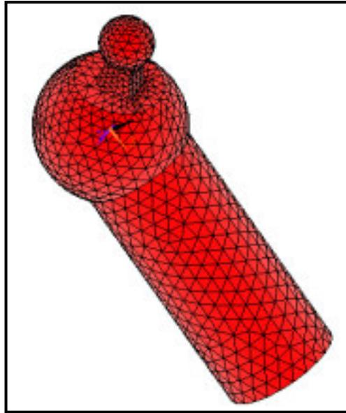
Figure 6.7 - The meshed volumes of all three components of the simplified cemented femoral system
