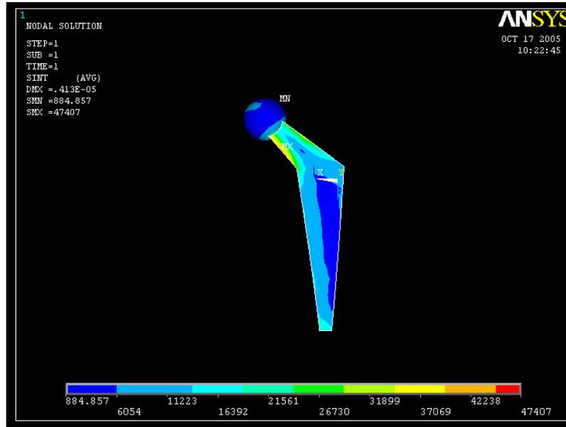
Figure 5.12 – The distribution of stress in the femoral stem in the un-cemented FEA in the z-x plane for 1 contact pair
