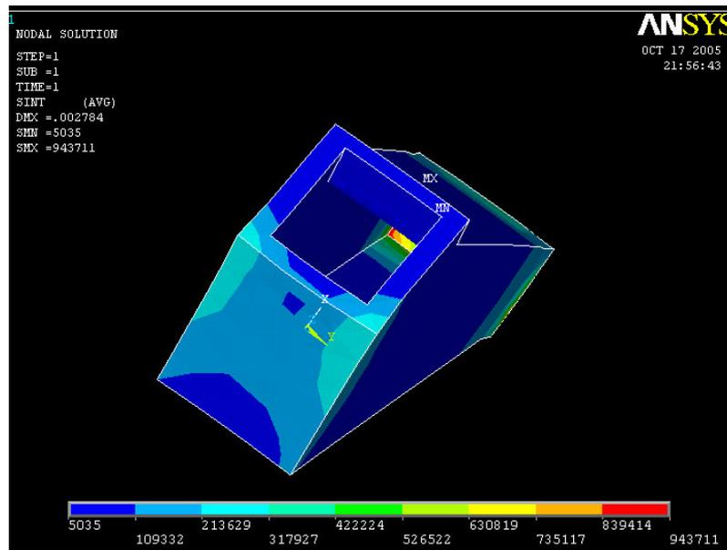
Figure 6.20 - View 2 of the distribution of stress in the cement for the second analysis for the cemented hip
