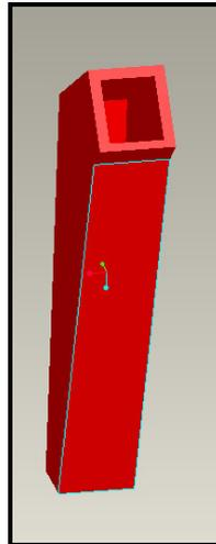
Figure 6.2 - The simplified cement volume used in the cemented hip analysis
