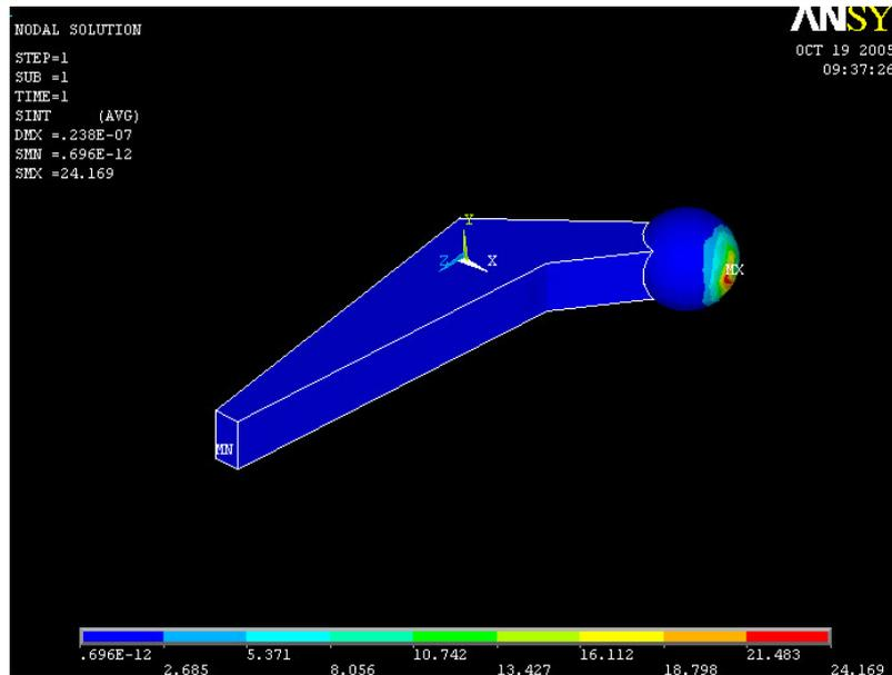
Figure 6.25 - The stress in the femoral stem for the third analysis of the cemented hip
