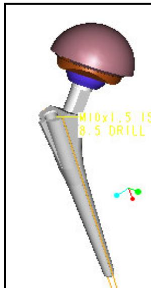
Figure 4.15 – The assembly created of the un-cemented hip
