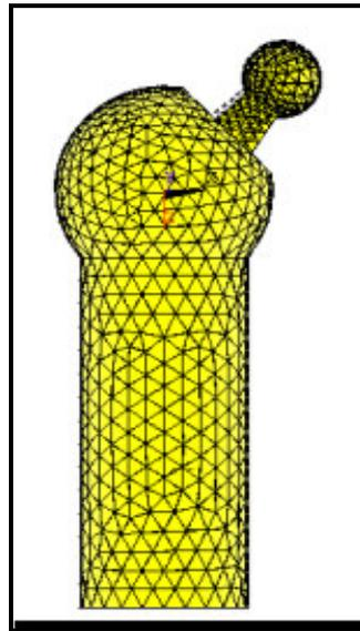
Figure 6.22 - The deformation for the third analysis done on the cemented hip in the z-x plane
