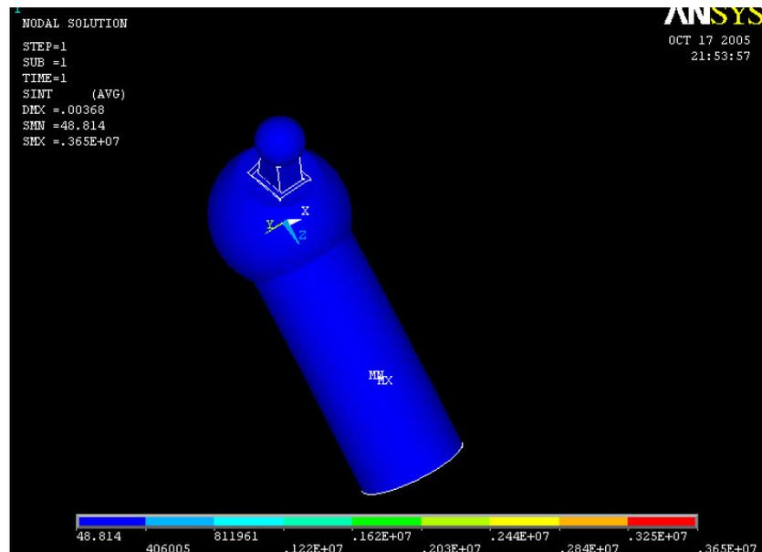
Figure 6.18 - The distribution of stress in the whole cemented hip for the second analysis
