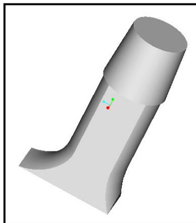
Figure 4.3 - The femoral neck for the cemented prosthesis
