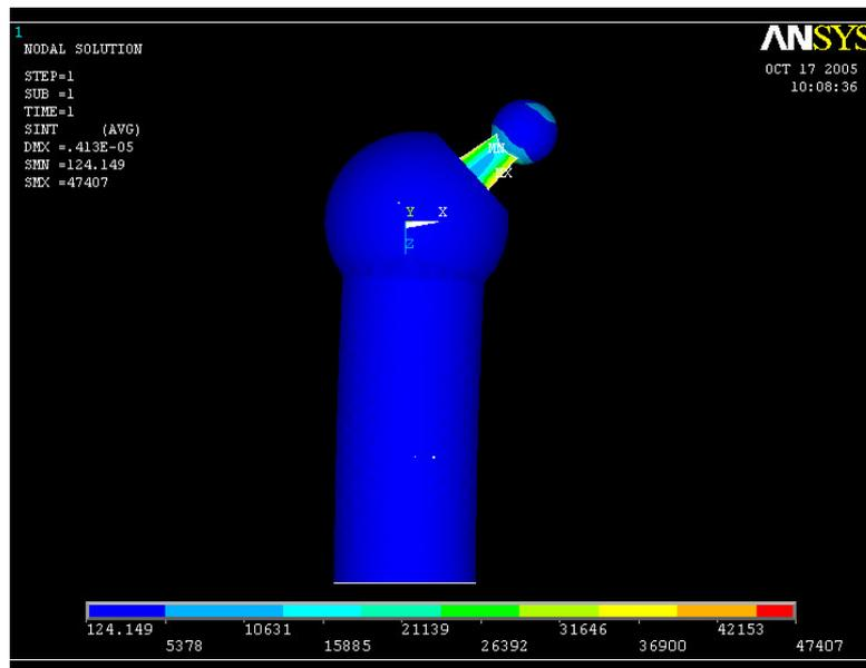
Figure 5.10 – The stress intensity in the un-cemented hip components in the z-x plane for 1 contact pair
