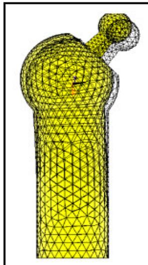
Figure 6.16 - The deformation of the cemented hip in the z-x plane
