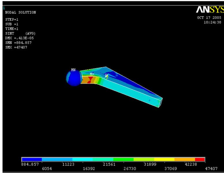
Figure 5.14 – An isometric view of the femoral stem showing the stress on the medial side for 1 contact pair
