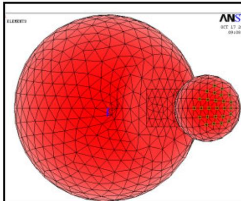
Figure 5.6 – The nodes selected on the femoral head for the application of loading
