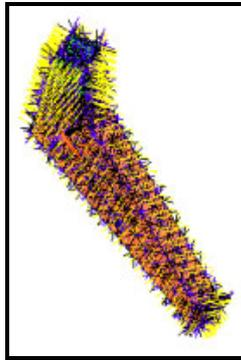
Figure 6.9 - The contact pair between the cement and the femoral stem
