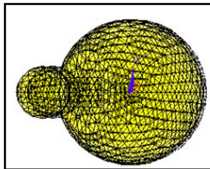
Figure 5.16 – The deformed and undeformed shape of the un-cemented hip in the x-y plane with 2 contact pairs
