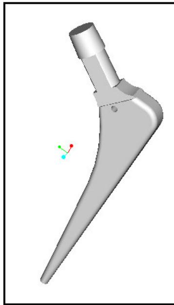
Figure 4.2 - The uncompleted cemented femoral stem created as one part
