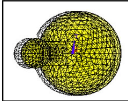
Figure 6.17 - The deformation of the cemented hip in the x-y plane
