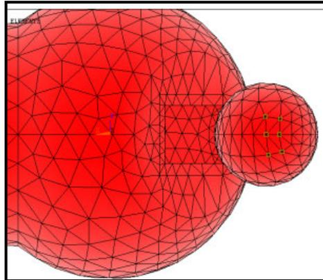
Figure 6.10 – The nodes on the femoral head that were constrained for the third analysis of the cemented hip
