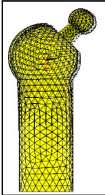
Figure 6.11 - The deformation in the z-x plane for the first analysis of the cemented hip
