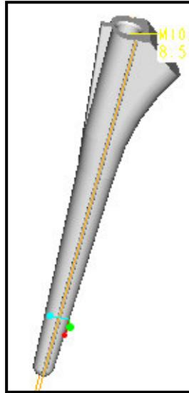
Figure 4.7 – The ProEngineer model created of the un-cemented femoral stem without the modular neck
