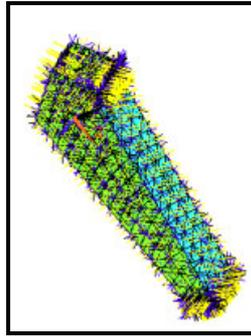
Figure 6.8 - The contact pair between the femur and the cement
