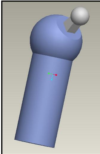
Figure 5.3 - The simplified assembly of the un-cemented femoral system
