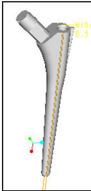
Figure 7.1 – The un-cemented femoral stem modelled in chapter 4
