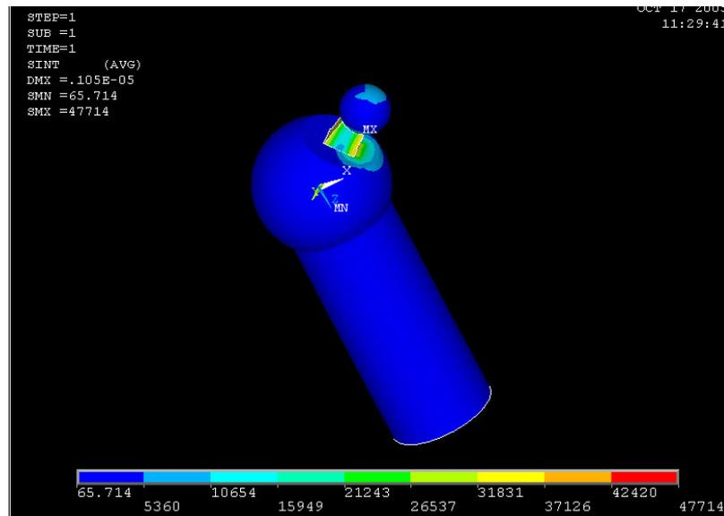
Figure 5.17 – The stress intensity of the un-cemented hip with 2 contact pairs
