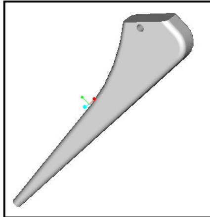
Figure 4.4 - The femoral stem for the cemented prosthesis
