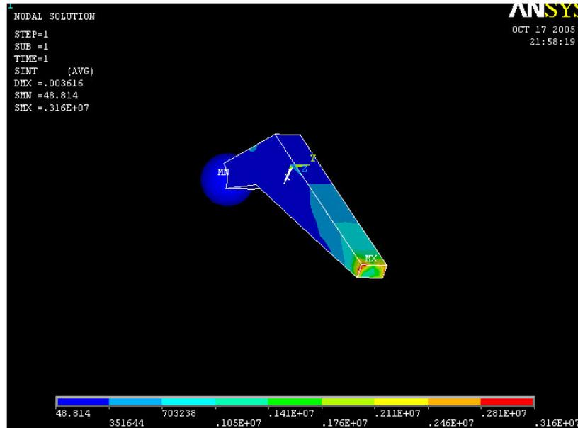
Figure 6.21 - The distribution of stress throughout the femoral stem for the second analysis of the cemented hip
