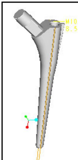
Figure 4.8 – The ProEngineer model created of the un-cemented femoral stem with the modular neck
