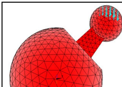
Figure 5.7 – The loading applied to the femoral head
