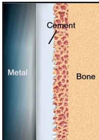
Figure 2.3 - The layers between the metal prosthesis and the bone in a cemented implant
