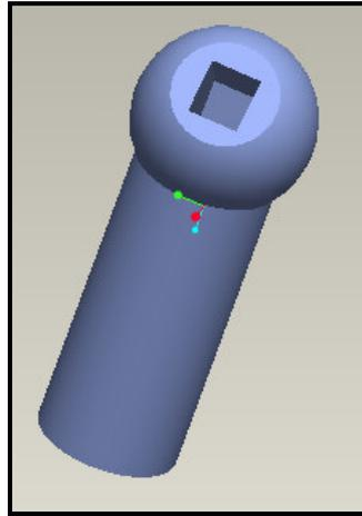
Figure 6.1 - The simplified femur that was created for the cemented analysis
