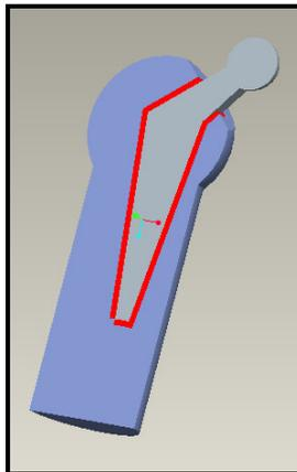
Figure 6.4 - A sectioned assembly of the simplified femoral system in ProEngineer
