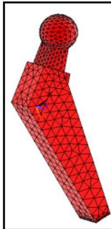
Figure 6.6 - The meshed volumes of the femoral stem and the cement
