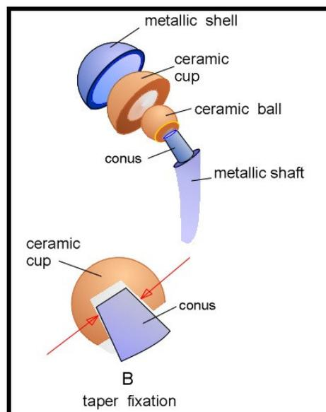
Figure 2.1 - Ceramic on ceramic hip prosthesis
