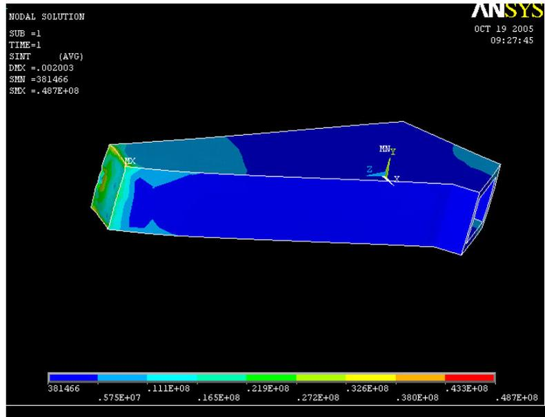
Figure 6.13 – View 1 of the stress distribution in the cement for the first cemented hip analysis
