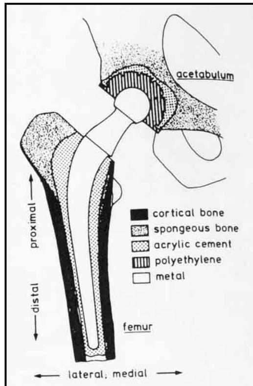
Figure 1.5 - Cross section of a cemented THR
