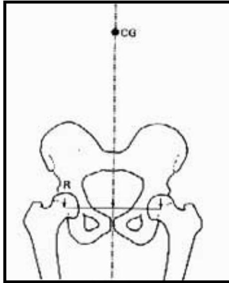
Figure 2.5 - Schematic showing the direction and magnitude of the load on the femoral head in symmetrical two-leg stance
