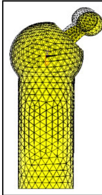
Figure 5.15 – The deformed and undeformed shape of the un-cemented hip in the z-x plane with 2 contact pairs
