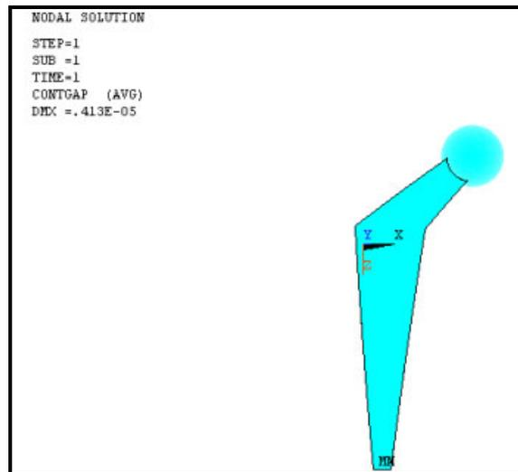
Figure 5.20 - The non-existent contact pressure on the un-cemented femoral stem
