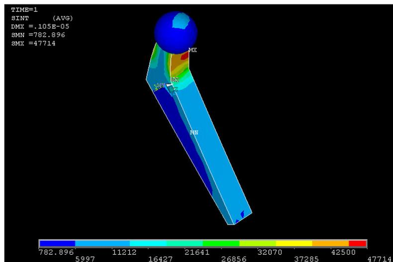
Figure 5.18 – View 1 of the stress intensity through the femoral stem for the un-cemented hip with 2 contact pairs
