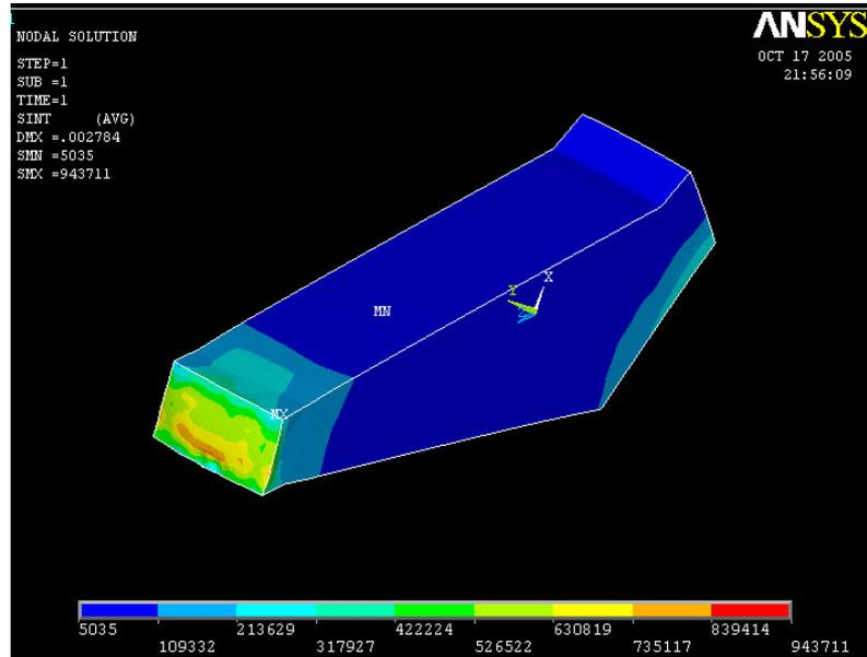
Figure 6.19 - View 1 of the distribution of stress in the cement for the second analysis of the cemented hip
