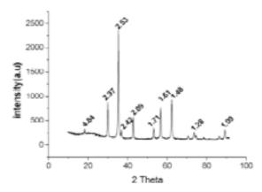
Fig. 1: X-ray diffraction of MNPs.
