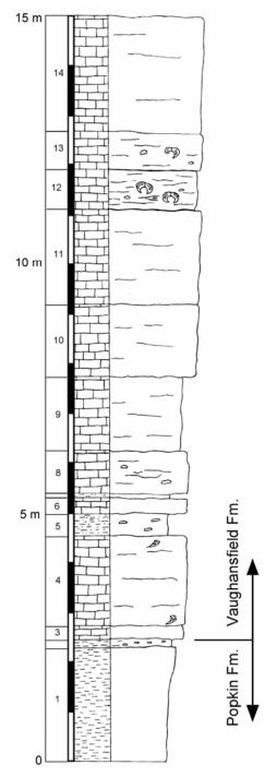
Figure 6. Graphic log of the Vaughansfield Formation stratotype in the vicinity of Flamstead. See Figure 2 for key.
