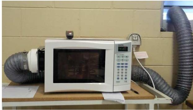
**Figure 11:** Microwave that was used to post cure the samples
