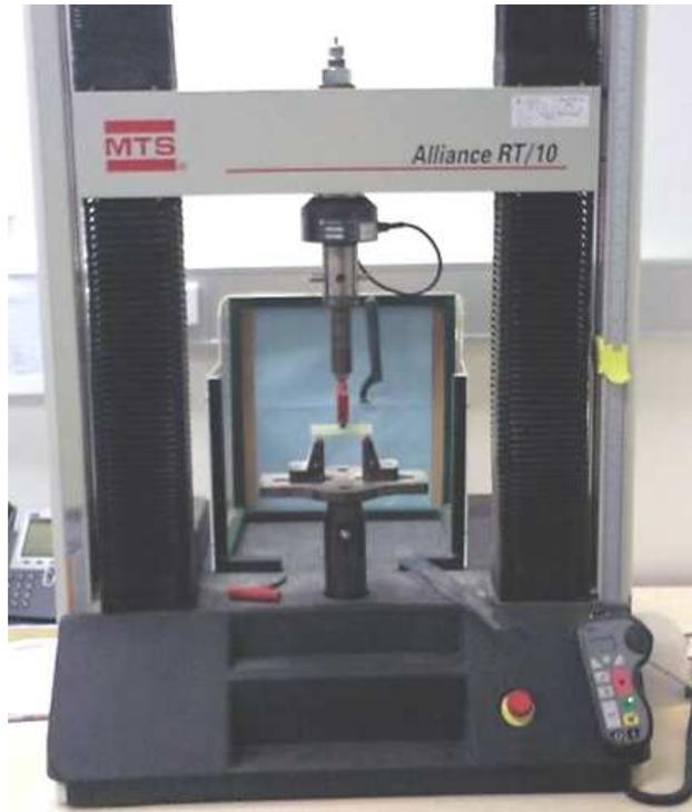
**Figure 17:** 10kN MTS Machine
