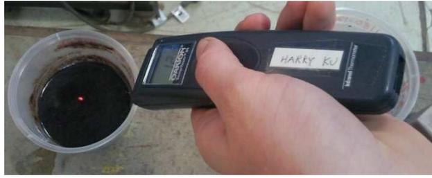
**Figure 10:** Measuring the temperature of the epoxy sample with an infrared thermocouple
