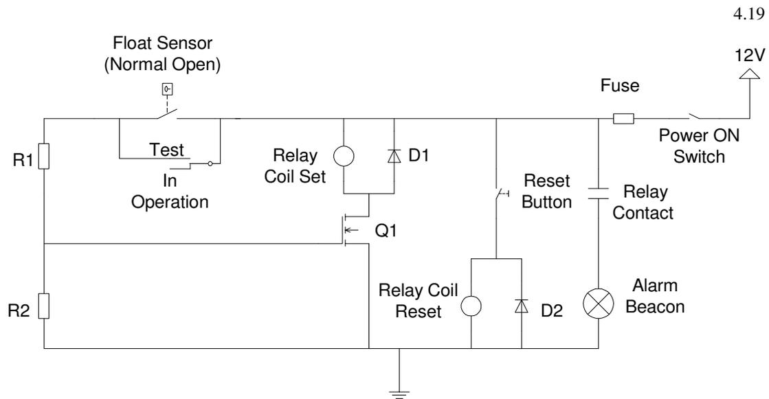
Fig 4.14 Normally Open Float Sensor Circuit Design
