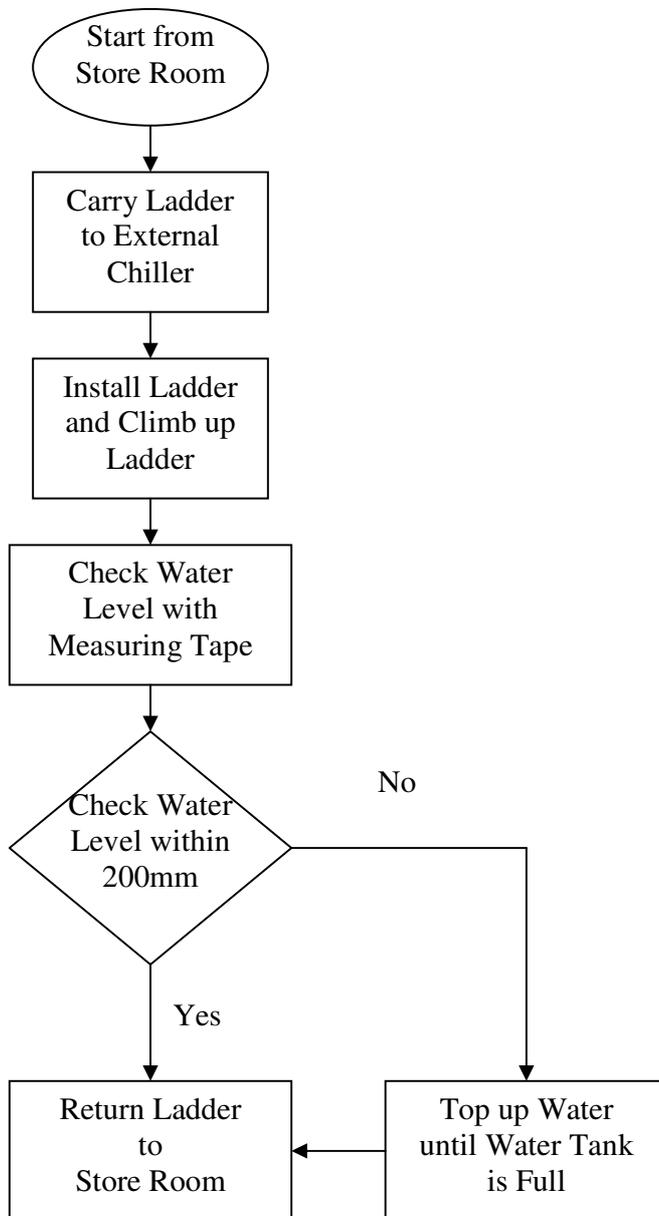
Fig 2.3 Water Level Monitoring Flow Chart
