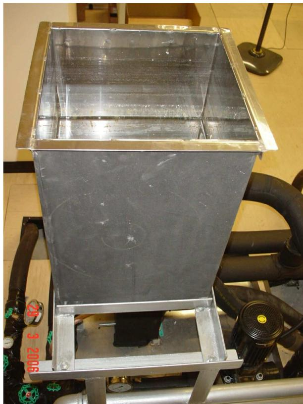
Fig 2.1 Top View of the Water Tank in the External Chiller
