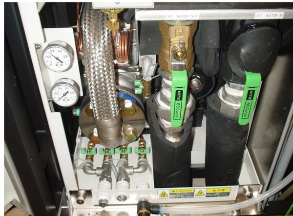
Fig. 5.6 Tester Chiller Unit Water Pan
