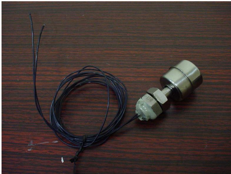
Fig 4.10 Vertical Float Sensor
