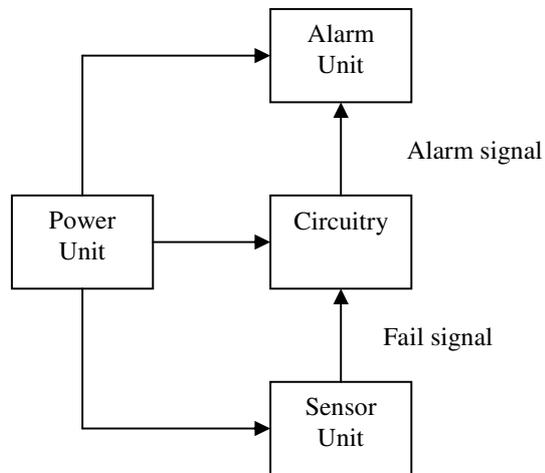
Fig. 4.6 Simplified Block Diagram of the Water Level Detection Jig
