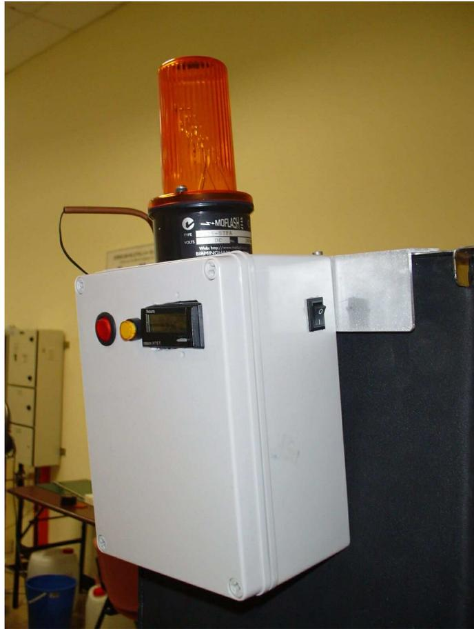
Fig 4.24 Water level detection jig attached to the water tank
