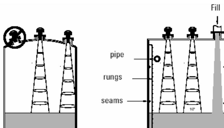
Fig 4.9 Location of the Ultrasonic Sensor
