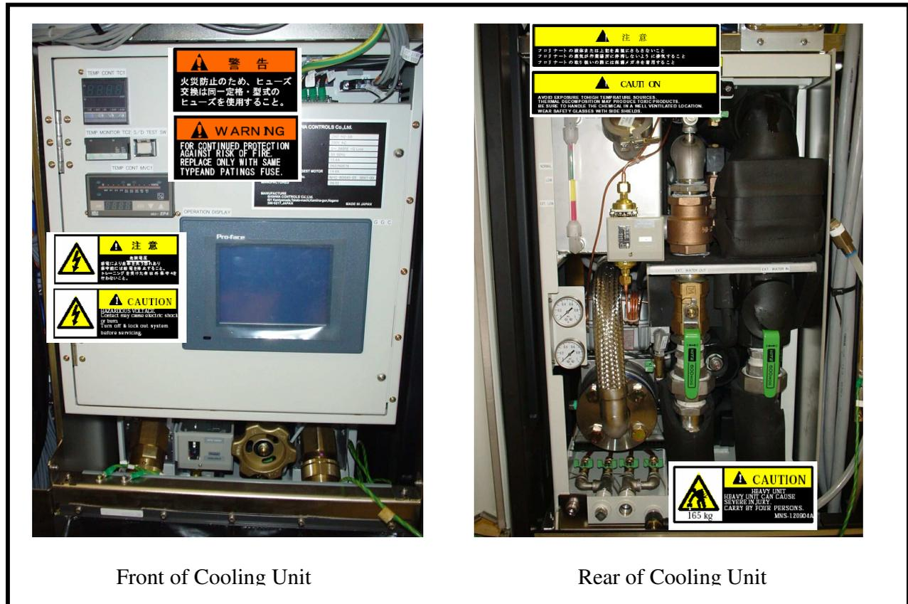
Fig 6.5 Location of warning labels in the cooling unit
