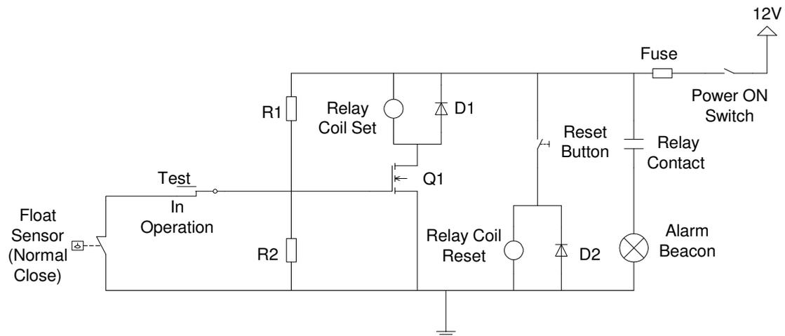
Fig 4.15 Normally Close Float Sensor Circuit Design
