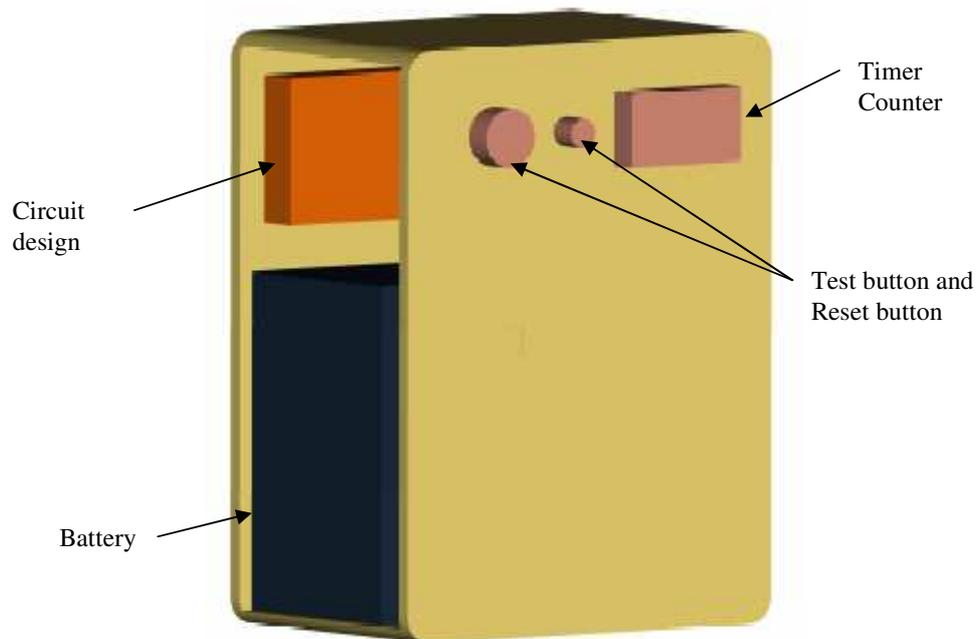
Fig 4.19 Control Box layout
