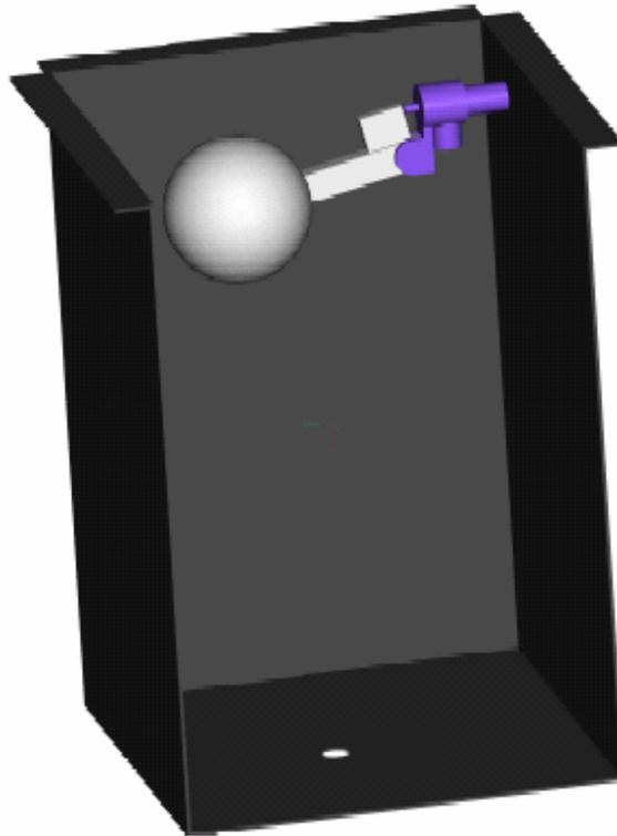
Fig. 4.1 Toilet Flush System attached to the water tank
