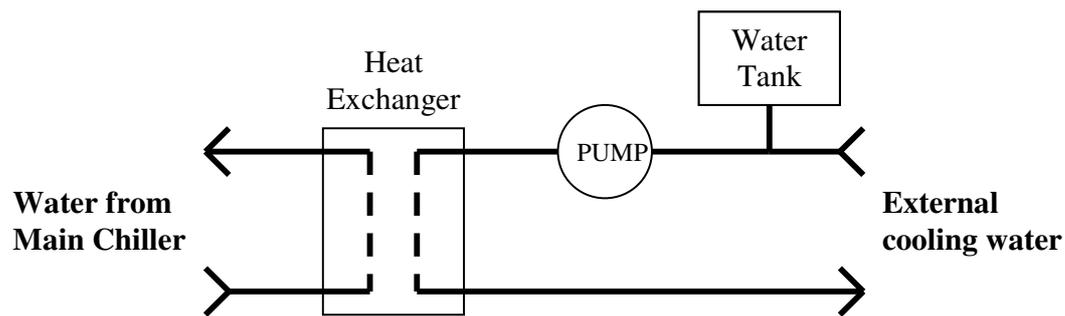
Fig 1.7 Simplified Block Diagram of the External Chiller
