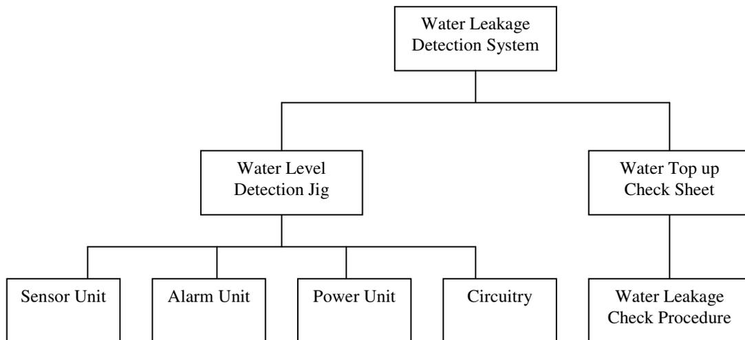
Fig 4.5 Hierarchy of the Water Leakage Detection System
