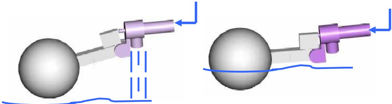
Fig. 4.2 Float position at different water level height
