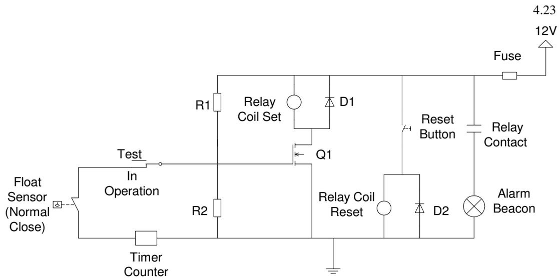
Fig 4.16 Timer counter added into the normally close circuit
