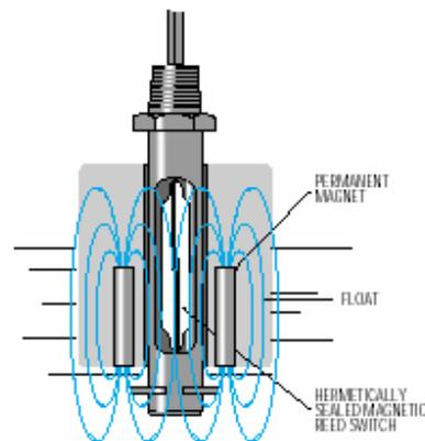
Fig 4.8 Drawing of a typical Vertical Float Sensor
