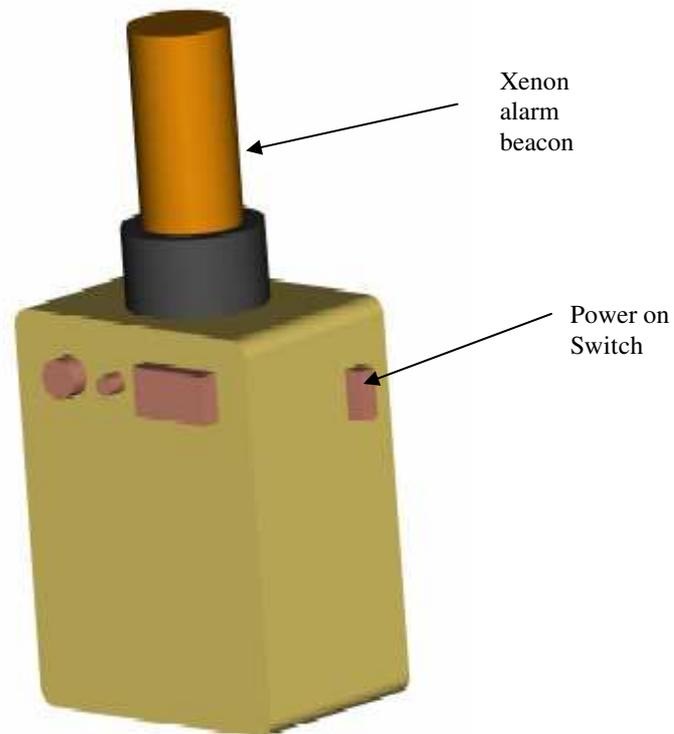
Fig 4.20 Control box with xenon alarm beacon attached
