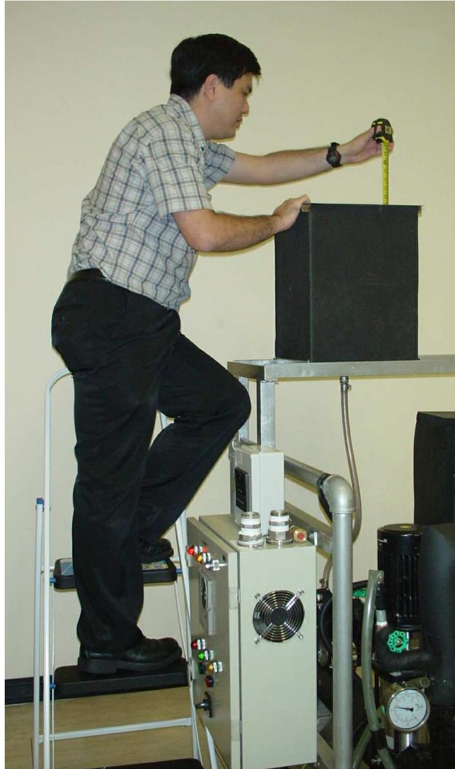
Fig 2.2 Monitoring the water level in the water tank
