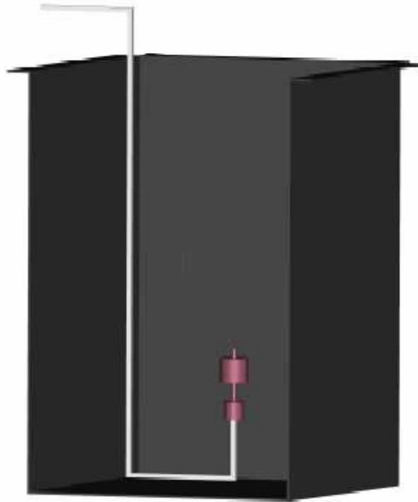
Fig 4.17 Float sensor placed vertically in the water tank
